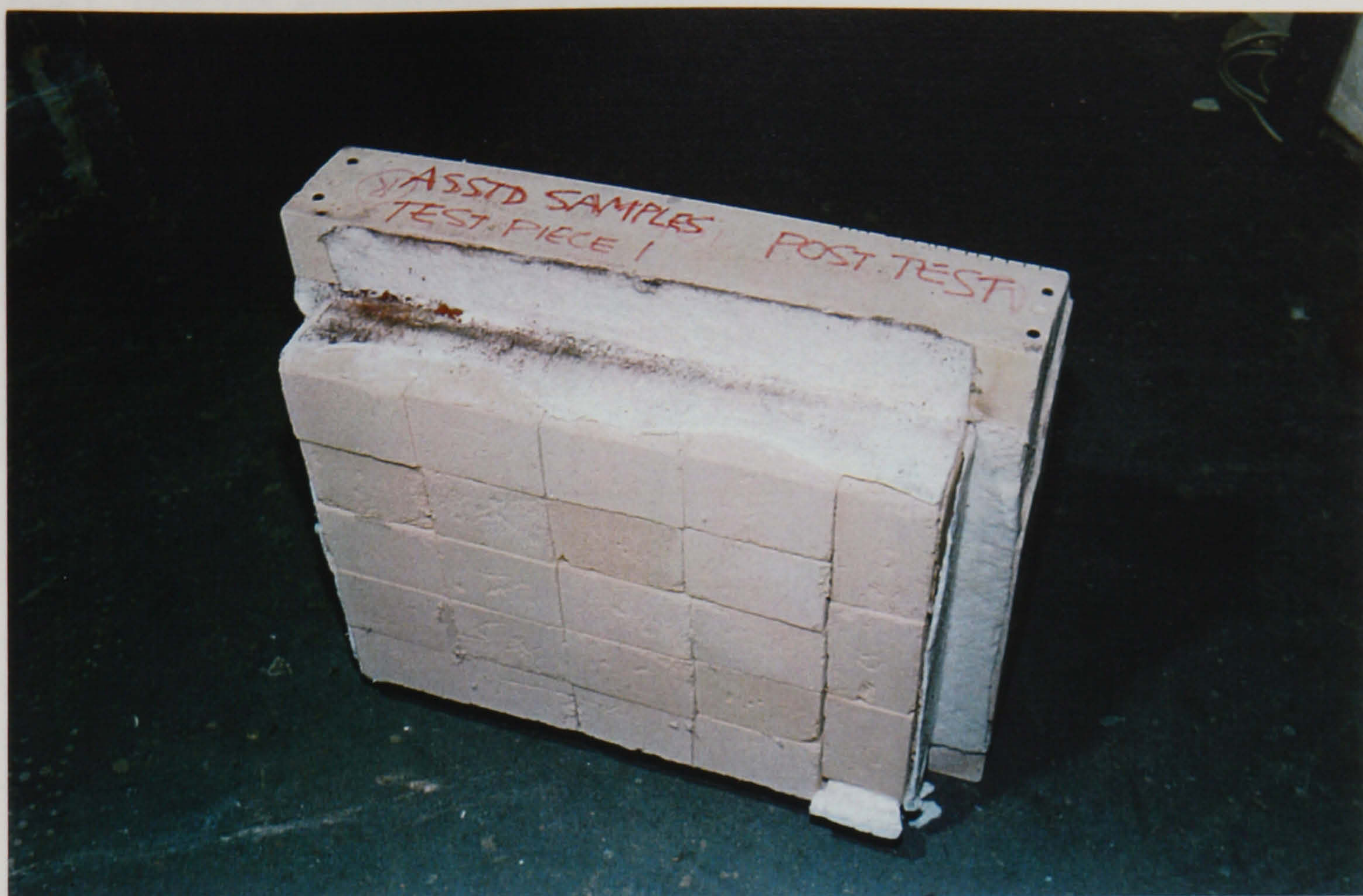
Figure A.5.9 Post test condition of assorted Insuline samples
