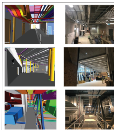
Image 2: Synchronized MEP BIM model applying MagiCAD (Case Study Project).
