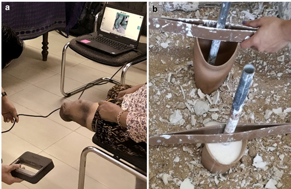
Fig. 1 A 3D scanning a participant's residual limb, and B creating alginate moulds of the sockets
