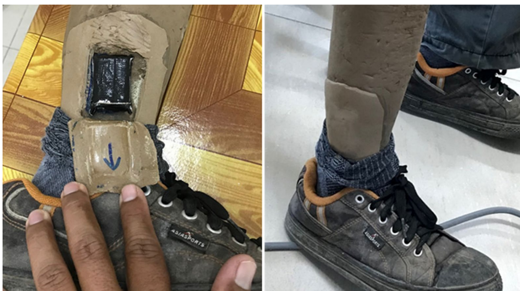
Fig. 2 Embedding the accelerometer in the prosthetic cosmesis. A new cosmesis was made and provided following study completion
