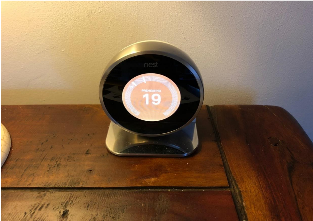
Image 9. 'Smart' digital thermostats, such as the 'Nest' shown here, are becoming commonplace now. This may be considered a standard feature for time and temperature control in a typical UK home.
