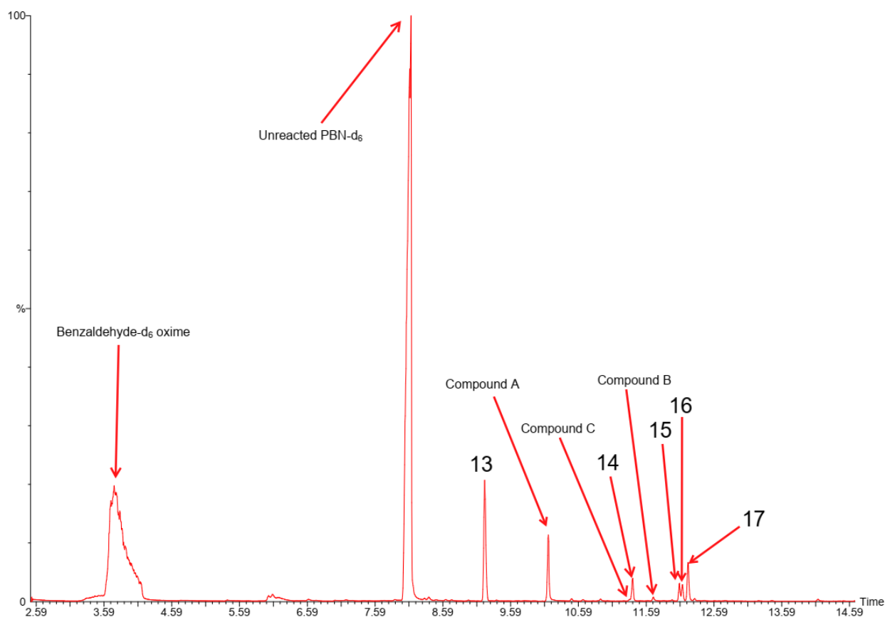
Figure 5.1.3 The total ion chromatogram obtained from the GC-MS analysis of the Fenton system with PBN-d 6 in the presence of 3-methyl butanal
