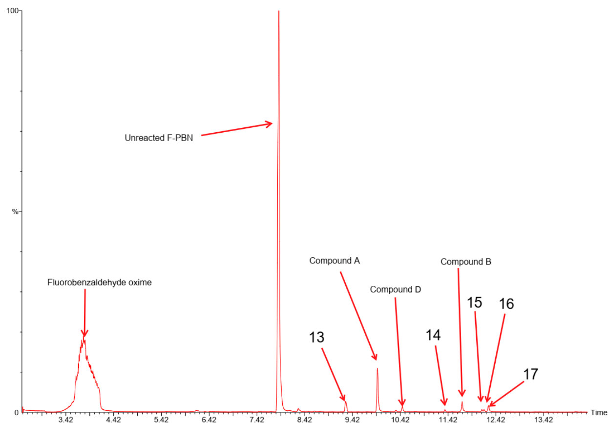
Figure 5.1.5 The total ion chromatogram obtained from the GC-MS analysis of the Fenton system with F-PBN in the presence of 3-methyl butanal
