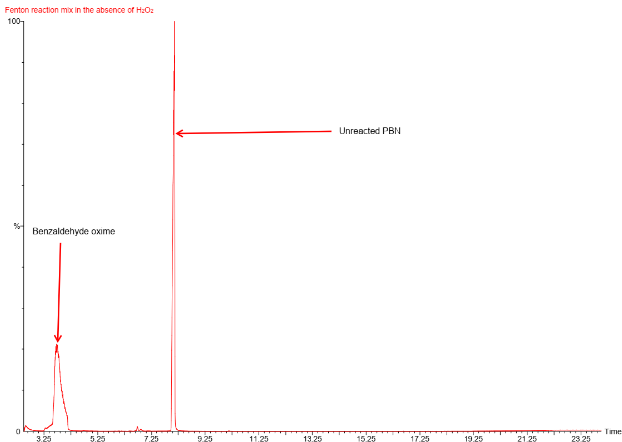
Figure 2.7.2 The total ion chromatogram obtained from the GC-MS analysis of the Fenton system with PBN in the absence of \text{H}_2\text{O}_2
