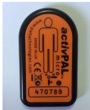
Figure 2.3: The activPAL™ micro accelerometer, with the figure on the front indicating the direction of attachment
