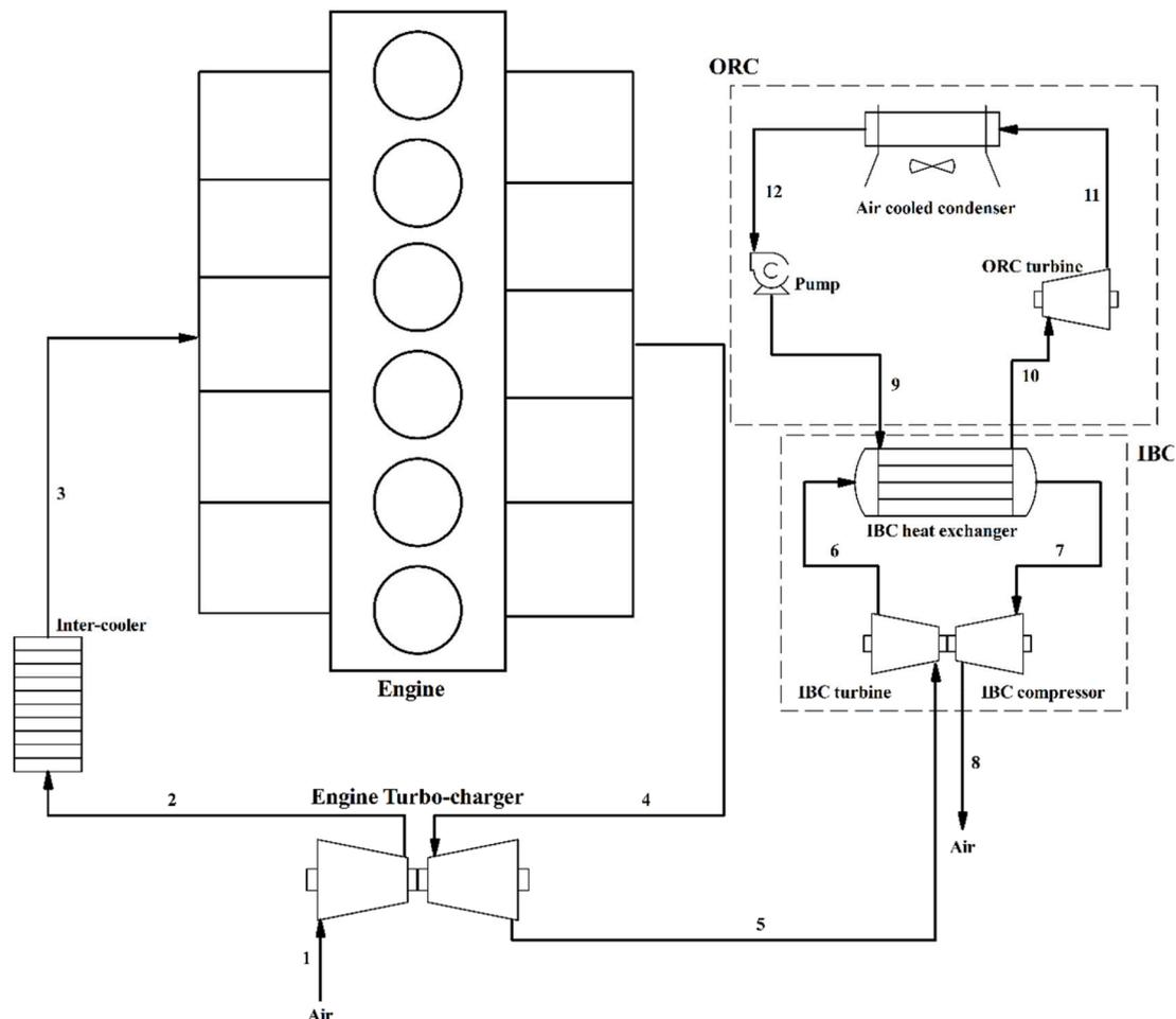
Fig. 1. The block diagram of the proposed system.
