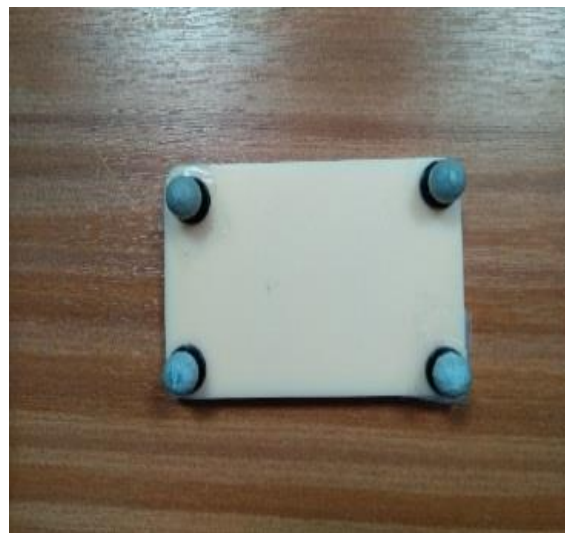
Figure 3-3 Marker cluster plates (with four nonlinear reflective markers)
