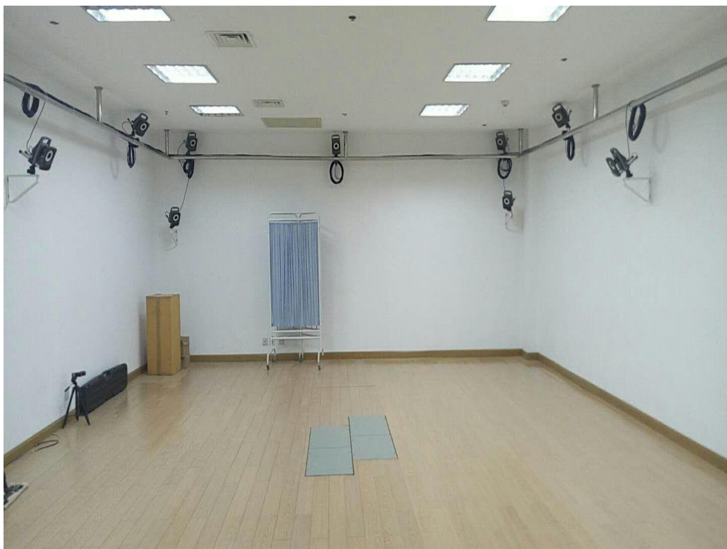
Figure 3-1 VICON motion analysis system in the gait laboratory of Shuguang Hospital affiliated to the Shanghai University of TCM
