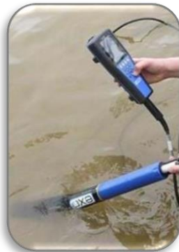
Figure 3. 15: The EXO3 Multiparameter Sonde- YSI
