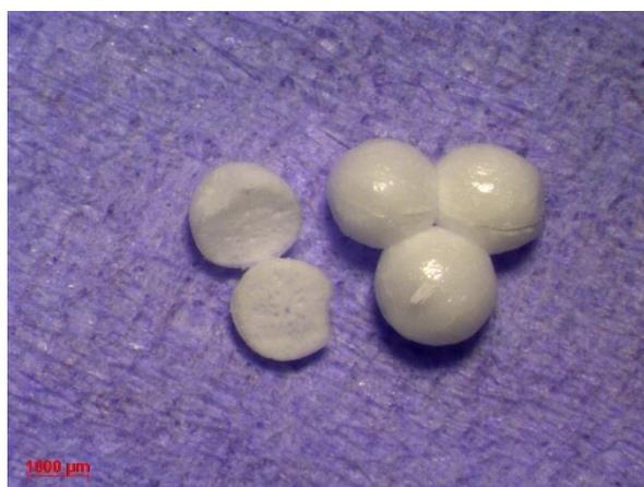
**Figure 4.105** Light micrograph of PSF NaBH<sub>4</sub> microcapsules - sample 47
