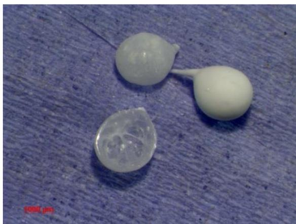
**Figure 4.76** Light micrograph of PSF  $\text{Li}_3\text{PO}_4$  microcapsules - sample 30
