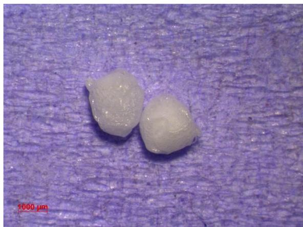
**Figure 4.101** Light micrograph of PSF NaBH<sub>4</sub> microcapsules - sample 45
