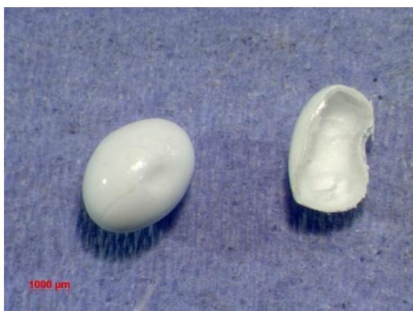
**Figure 4.59** Light micrograph of PSF  $\text{Li}_2\text{CO}_3$  microcapsule - sample 20
