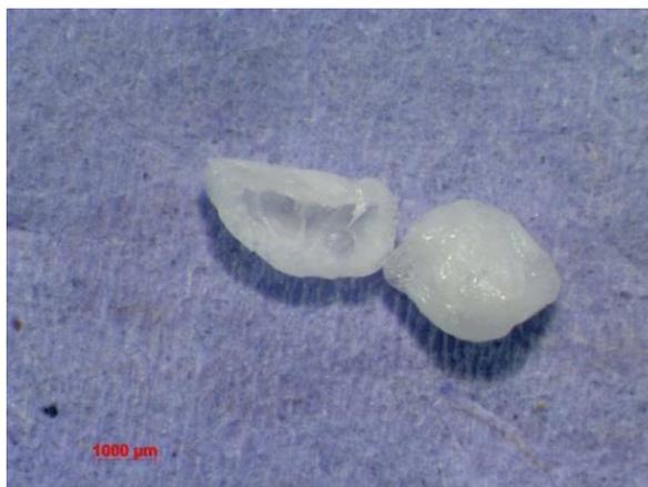
**Figure 4.61** Light micrograph of PSF  $\text{Li}_2\text{CO}_3$  microcapsule - sample 22
