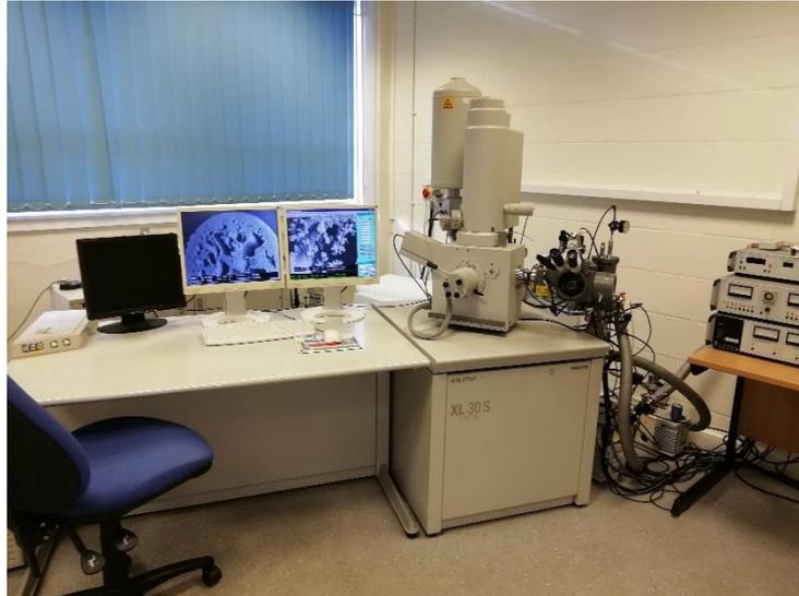
**Figure 3.2** Philips XL30 SFE Scanning Electron Microscope
