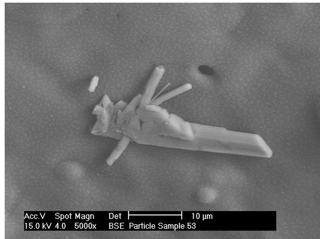
**Figure 4.131** SEM micrograph of internal area showing  $\text{NaBH}_4$  particles - sample 53
