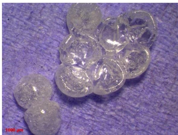
***Figure 4.111*** Light Micrograph of PSF NaBH<sub>4</sub> microcapsules - sample 48
