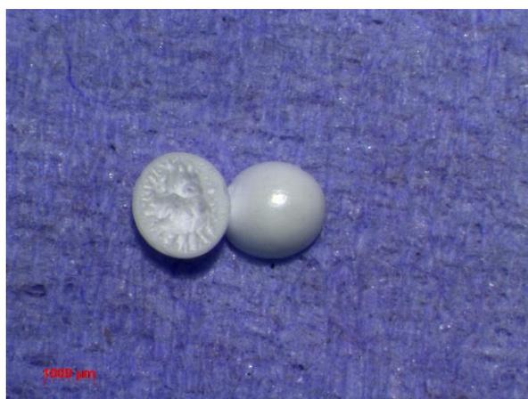
**Figure 4.94** Light micrograph of PSF LiNH<sub>2</sub> microcapsule - sample 39
