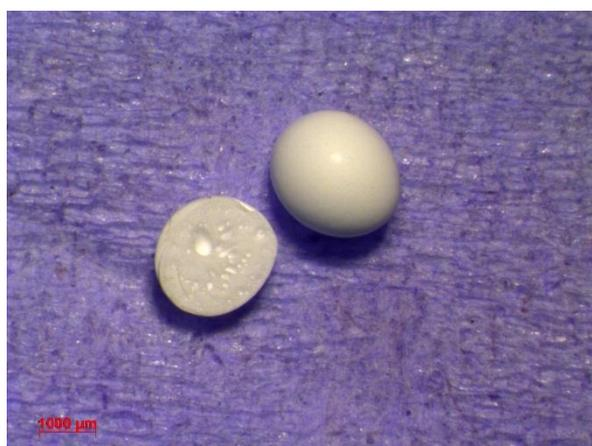
**Figure 4.102** Light micrograph of PSF NaBH<sub>4</sub> microcapsules - sample 46
