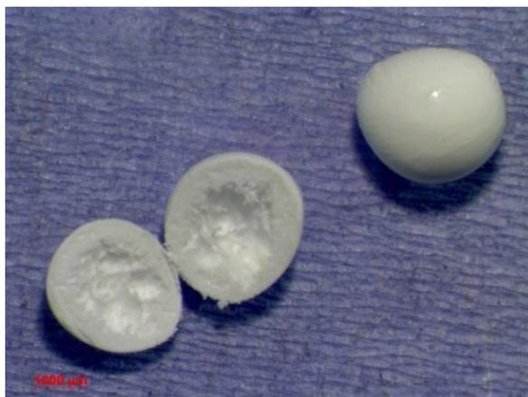
**Figure 4.69** Light micrograph of PSF  $\text{Li}_3\text{PO}_4$  microcapsules - sample 28
