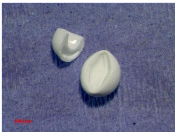
**Figure 4.68** Light micrograph of PSF  $\text{Li}_2\text{CO}_3$  microcapsules - sample 27
