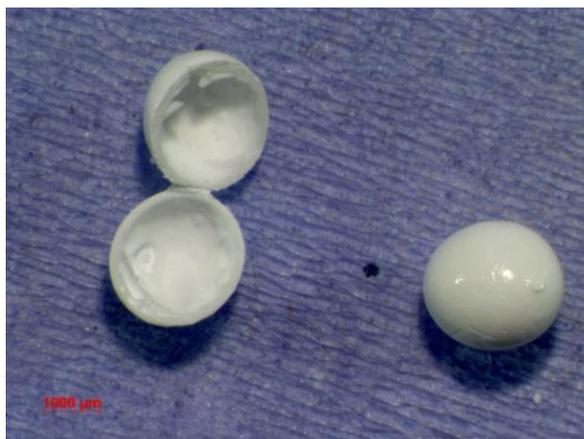
**Figure 4.65** Light micrograph of PSF  $\text{Li}_2\text{CO}_3$  microcapsules - sample 26
