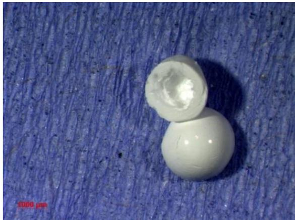
**Figure 4.58** Light micrograph of PSF  $\text{Li}_2\text{CO}_3$  microcapsule - sample 19
