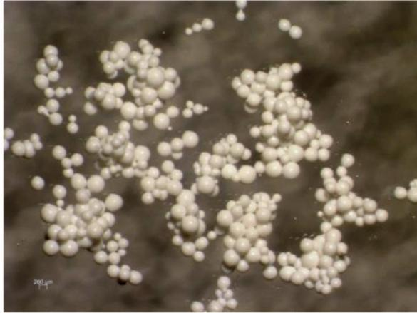
**Figure 4.5** Light micrograph of 1:2 ratio microcapsules
