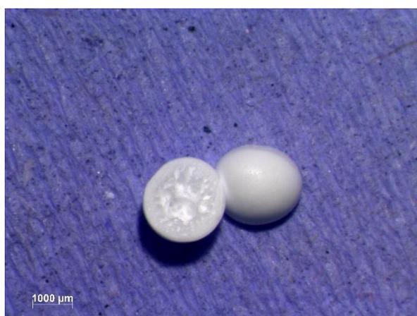
**Figure 4.92** Light micrograph of PSF-LiNH<sub>2</sub> microcapsule - sample 38
