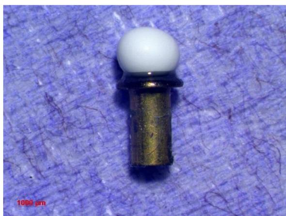
**Figure 4.117** Light micrograph of a glued microcapsule onto a brass rivet - sample 46
