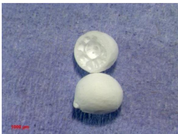
**Figure 4.64** Light micrograph of PSF  $\text{Li}_2\text{CO}_3$  microcapsule - sample 25
