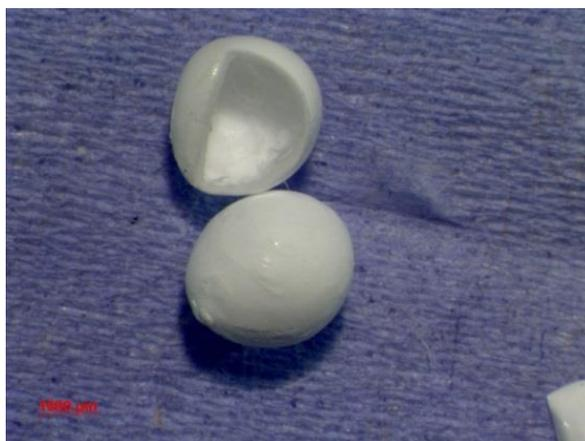
**Figure 4.72** Light micrograph of PSF  $\text{Li}_3\text{PO}_4$  microcapsules - sample 29
