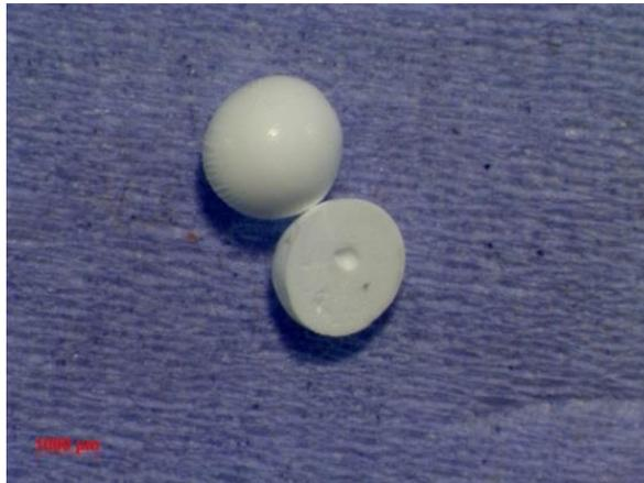
**Figure 4.79** Light micrograph of PSF  $\text{Li}_3\text{PO}_4$  microcapsule - sample 33
