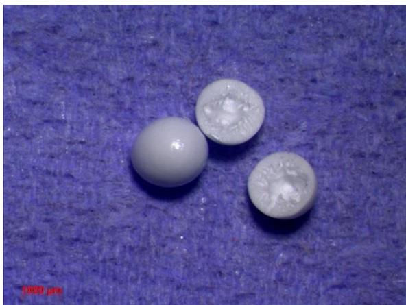
**Figure 4.99** Light micrograph of PSF NaBH<sub>4</sub> microcapsules - sample 43
