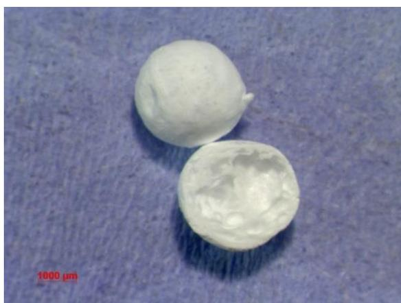
**Figure 4.62** Light micrograph of PSF  $\text{Li}_2\text{CO}_3$  microcapsule - sample 23
