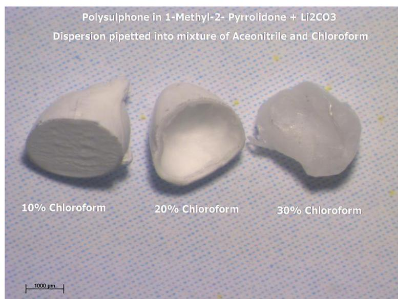
**Figure 4.67** Light micrograph of microcapsules from different solvent ratios
