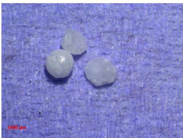
**Figure 4.97** Light micrograph of PSF  $\text{NaBH}_4$  microcapsules - sample 41
