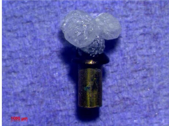
**Figure 4.122** Light micrograph of microcapsules glued onto a rivet using Loctite
