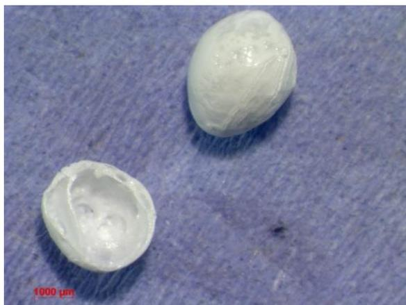
**Figure 4.63** Light micrograph of PSF  $\text{Li}_2\text{CO}_3$  microcapsule - sample 24
