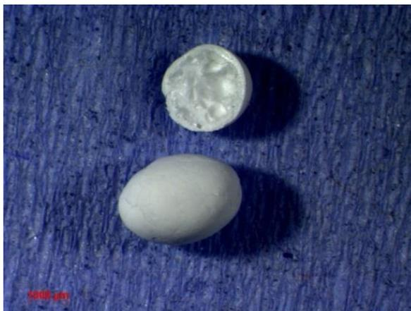
**Figure 4.57** Light micrograph of PSF-Li<sub>2</sub>CO<sub>3</sub> microcapsule - sample 18
