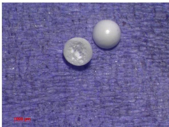
***Figure 4.98*** Light micrograph of PSF NaBH<sub>4</sub> microcapsule - sample 42
