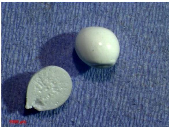
**Figure 4.56** Light micrograph of PSF  $\text{Li}_2\text{CO}_3$  microcapsules - sample 17
