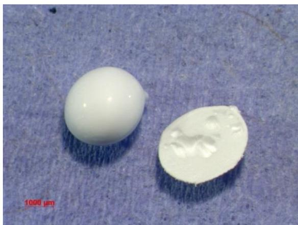
**Figure 4.60** Light micrograph of PSF  $\text{Li}_2\text{CO}_3$  microcapsule - sample 21
