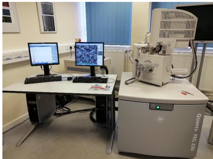
**Figure 3.1** FEI Quanta FEG 250 Scanning Electron Microscope
