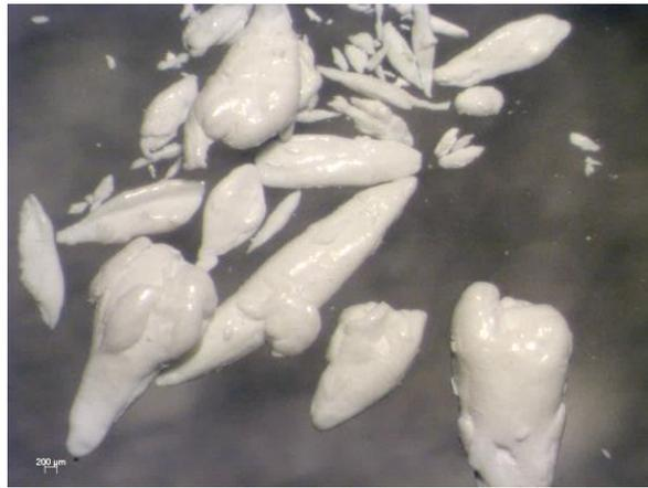
**Figure 4.3** Light micrograph of 2:1 ratio microcapsule
