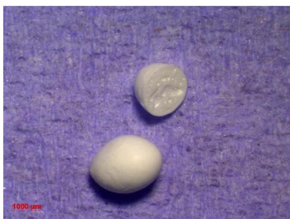
***Figure 4.112*** Light micrograph of PSF  $\text{NaBH}_4$  microcapsules - sample 49
