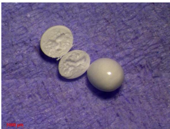
**Figure 4.113** Light micrograph of PSF NaBH<sub>4</sub> microcapsules - sample 50
