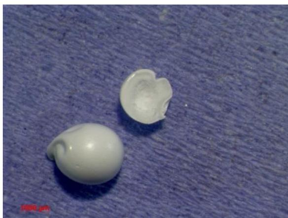
**Figure 4.77** Light micrograph of PSF  $\text{Li}_3\text{PO}_4$  microcapsules - sample 31
