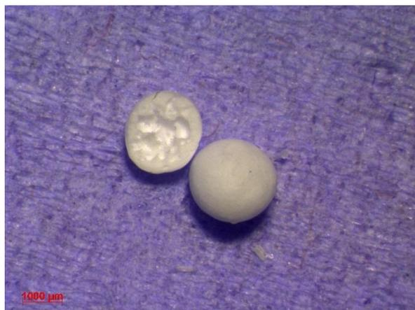
**Figure 4.115** Light micrograph of PSF  $\text{NaBH}_4$  microcapsules - sample 52
