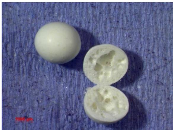
**Figure 4.86** Light micrograph of PSF LiNH<sub>2</sub> microcapsules - sample 36
