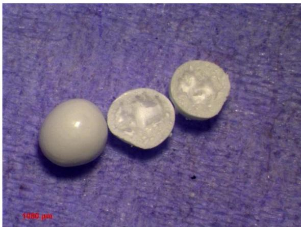
**Figure 4.114** Light micrograph of PSF  $\text{NaBH}_4$  microcapsules - sample 51
