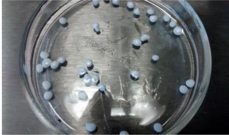
**Figure 4.18** Image of PSF polymer microcapsules
