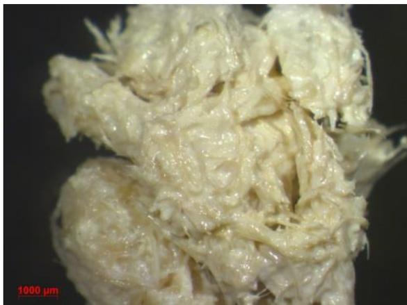
*Figure 4.9* Light micrograph of 1:2 ratio of CAP-TiO<sub>2</sub> using THF
