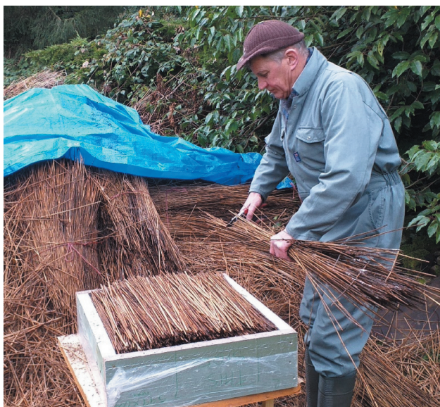
Figure 15. Preparing sample of original thatch removed from the roof for thermal conductivity testing. Image copyright Anthony Simpson.
