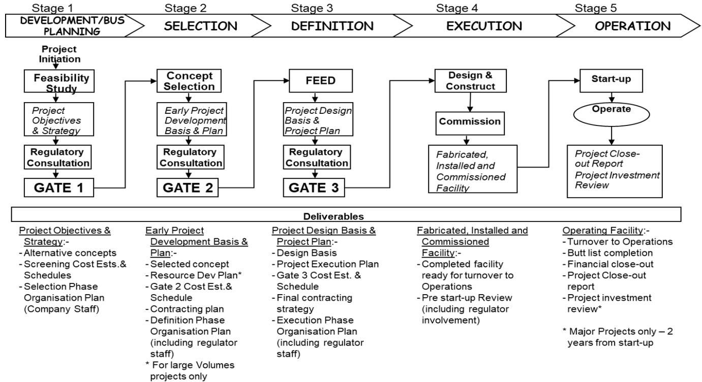
**FIGURE 2.4 The Five Stage-gate Project Phases (Lifecycle)**
