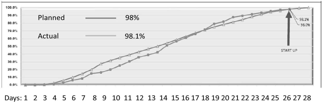
**Figure 4.19 Progress Schedule of Revamp Project Execution during Full Facility Shutdown.**
