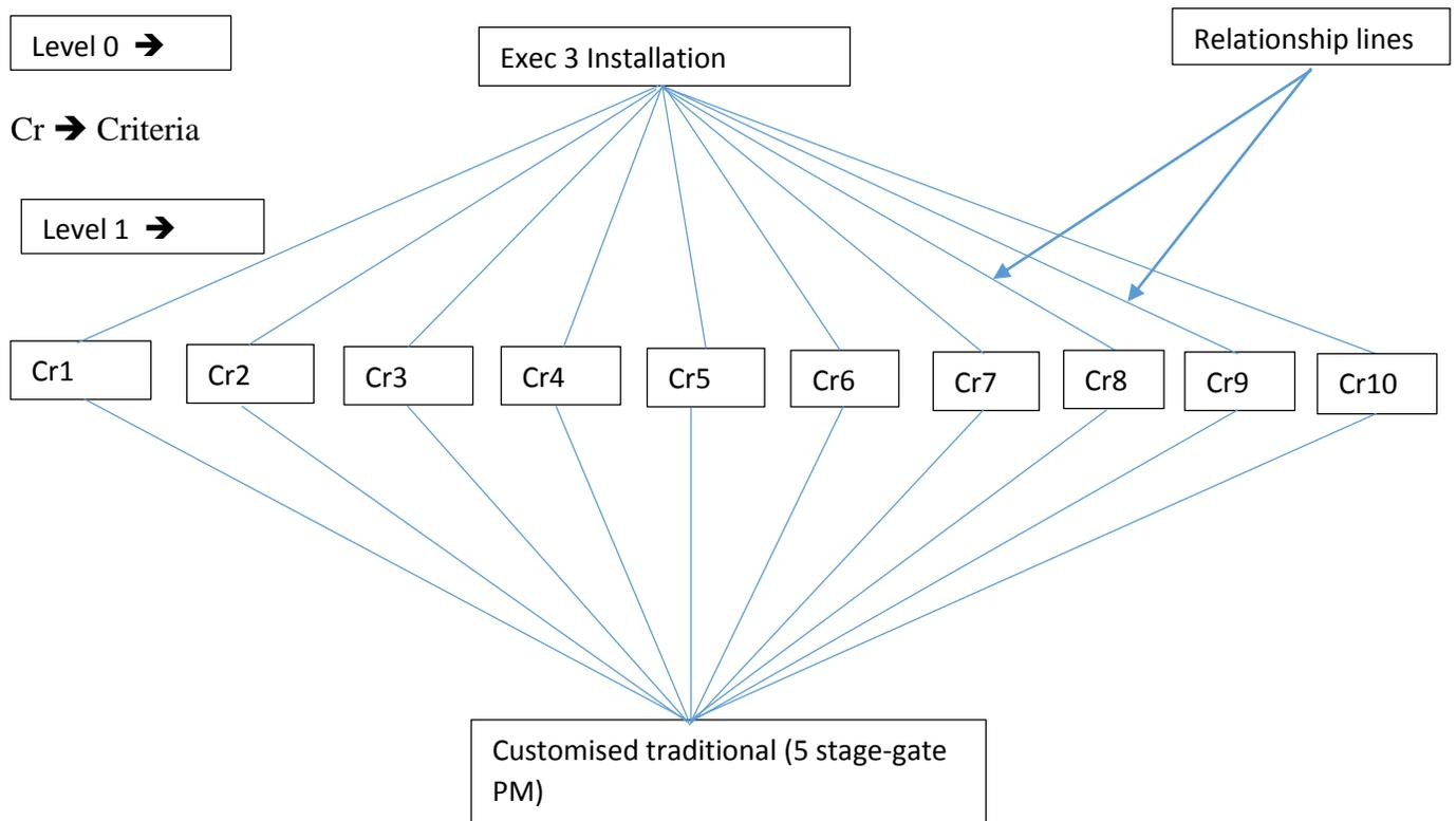
Figure 5.8 is indicative of the as-is installation model during the execution stage of FPSO revamp project realisation. The model is a typical three level, two step Analytic Hierarchy Process (AHP).
