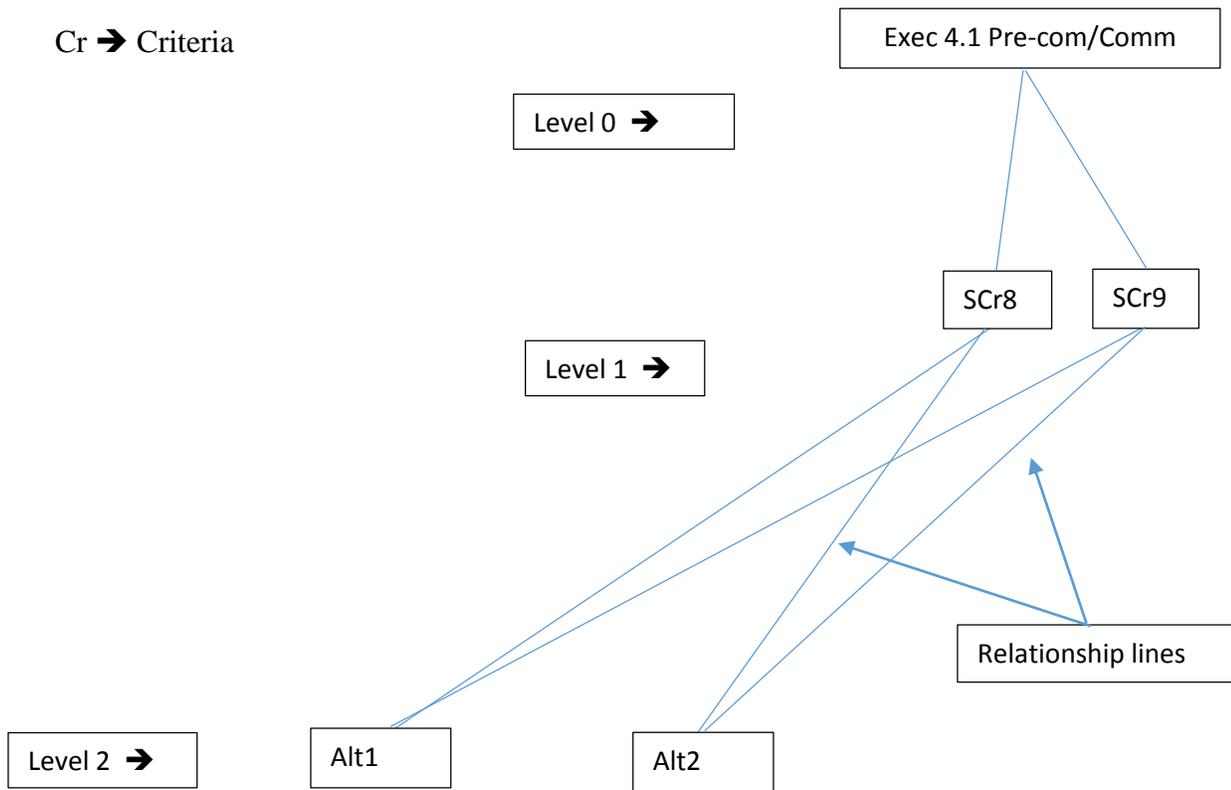
Figure 5.11 is indicative of the as-is Pre-com/Commissioning model during the execution stage of FPSO revamp project realisation. The model is a typical three level, two step Analytic Hierarchy Process (AHP). Exec 4Pre-com/Commissioning means execution stage 1 under the pre-commissioning/commissioning purview with a goal or objective function of detailed engineering optimisation at level zero (0).
