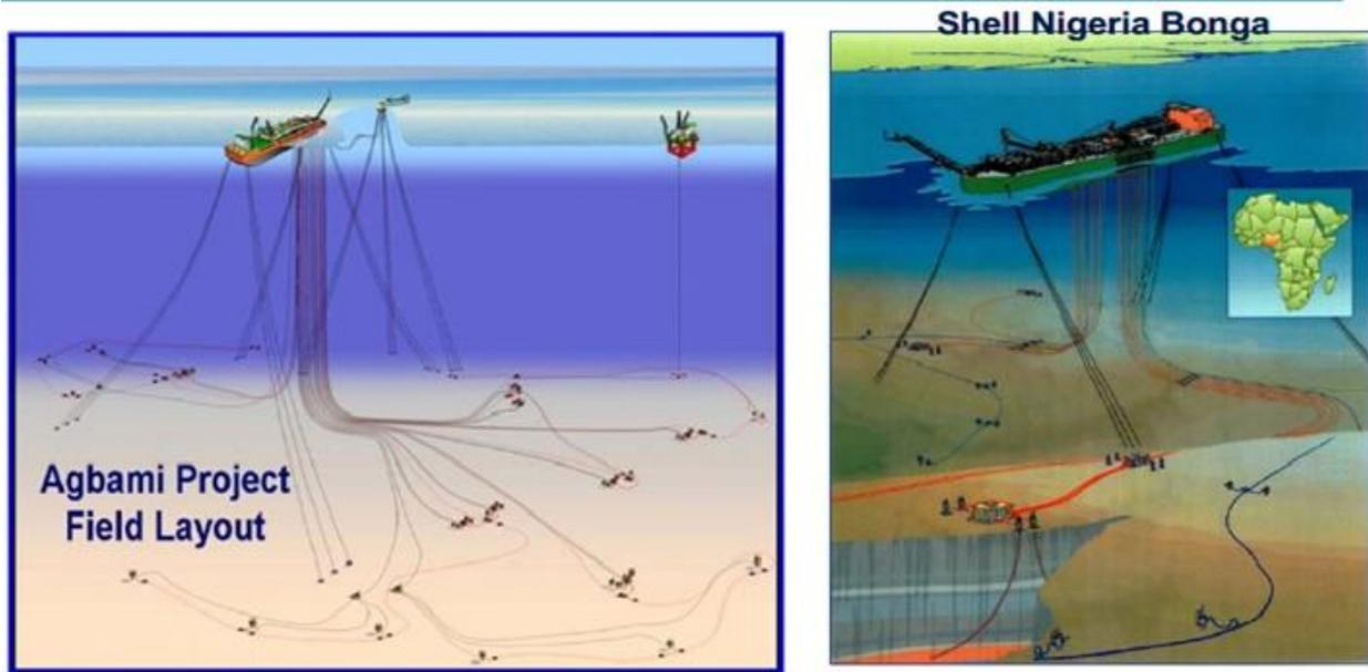
**FIGURE 2.9** Subsea UFR, and OLT connections to the FPSO
