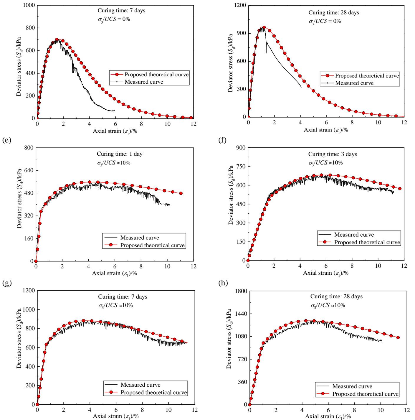
199 Fig.4 Comparison between experimental measurements and the proposed damage constitutive model predictions at different
