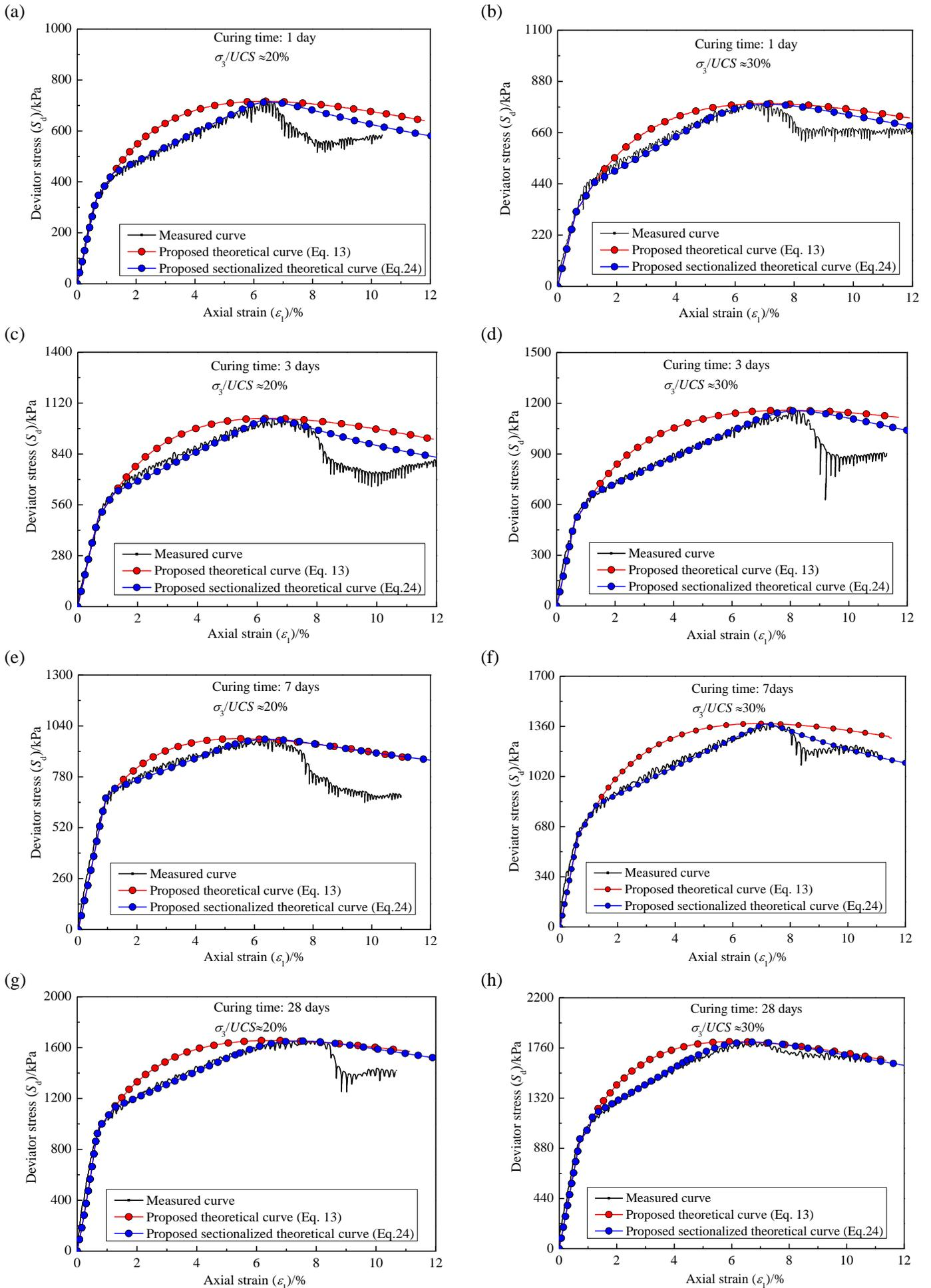
253 Fig. 7 Comparison between the theoretical stress-strain curves obtained by Eq. 24 & Eq. 13 and experimental curves of
