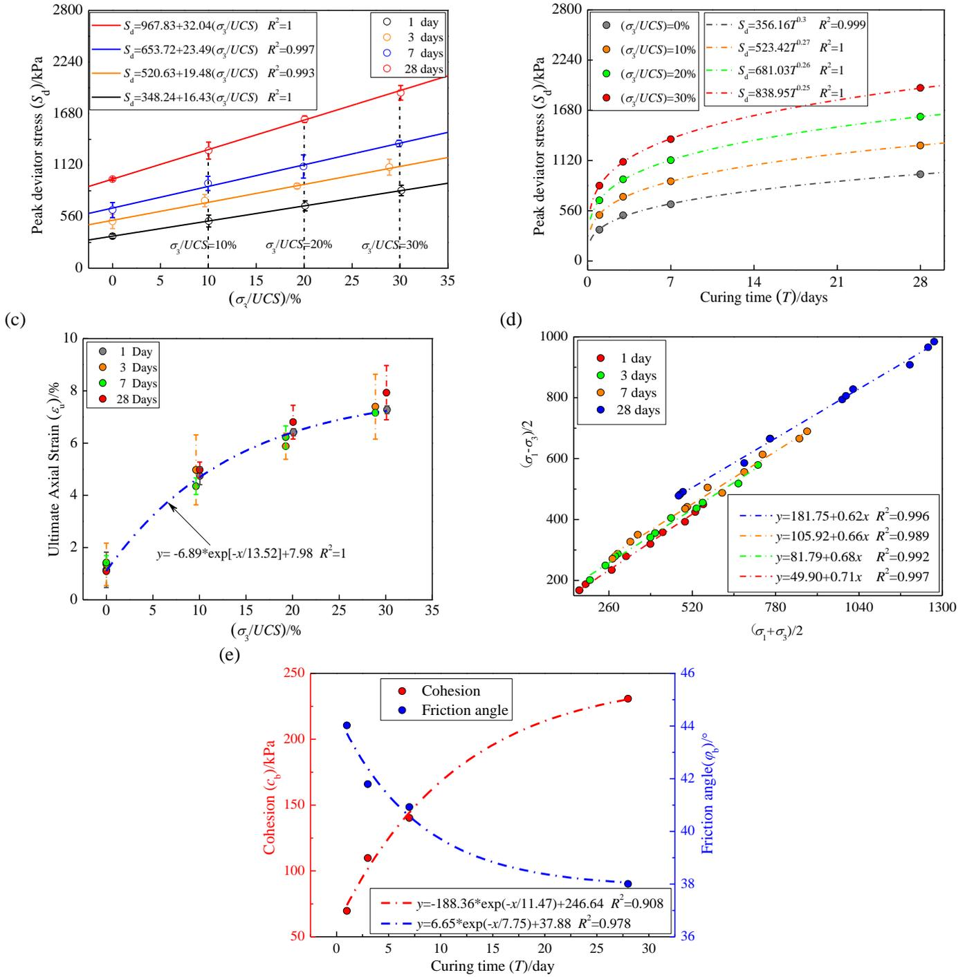
113 Fig. 3 The triaxial tested results of CPB samples under 4 different curing time (1, 3, 7, and 28 days) and 4 different lateral
