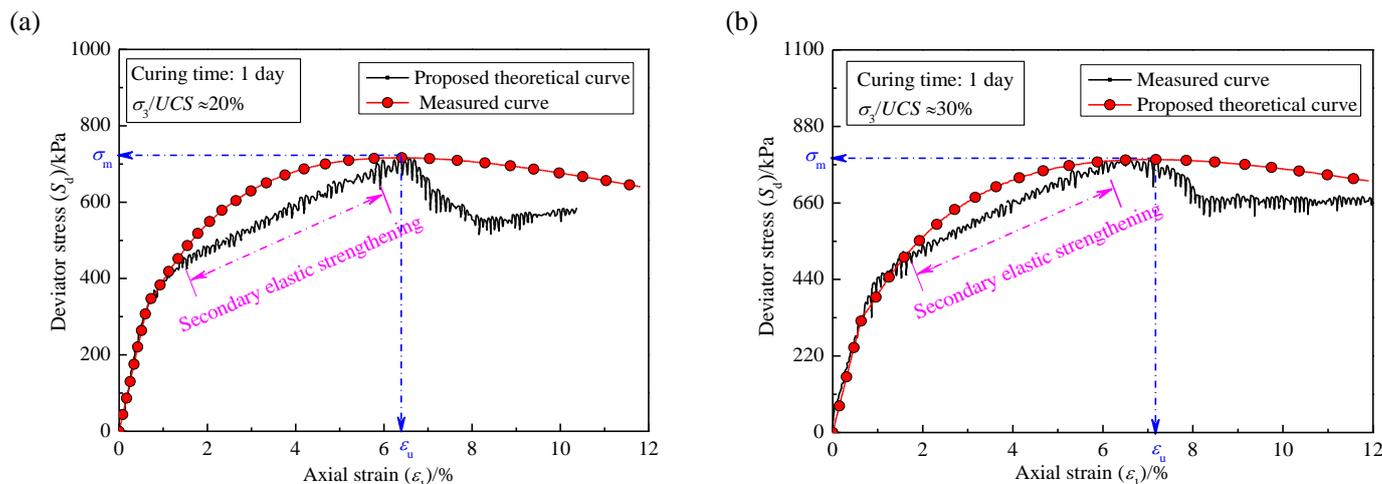
214 Fig. 5 Comparison between experimental and proposed theoretical curves of CPB with curing time of 1 day under
