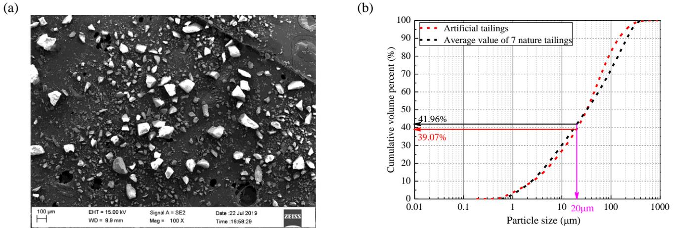
72 Fig.1 The relevant information about the mentioned tailings: (a) SEM image of AT (magnified 100 times); (b) the particle
