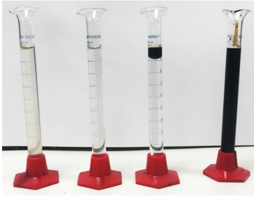
Figure 4.25: Effluents of Imbibition Experiment using Distilled Water
