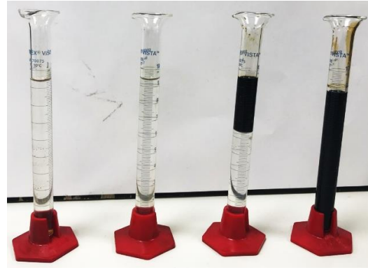
Figure 4.26: Effluents of Imbibition Experiment using 100,000ppm Cl Brine
