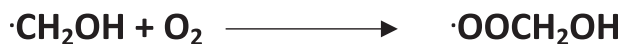
Scheme 4. Generation of the hydroxymethyl peroxy radical by addition of oxygen to the hydroxymethyl radical.
