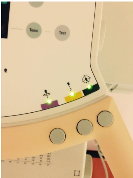
Figure 7 - Source to image receptor alignment indicators illuminated on x-ray tube housing
