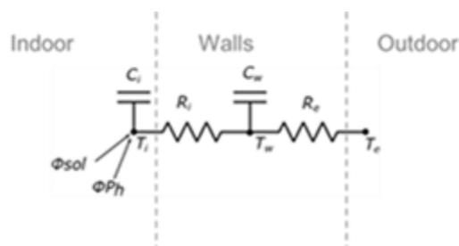
Figure 31. RC model example for adapted coheating
