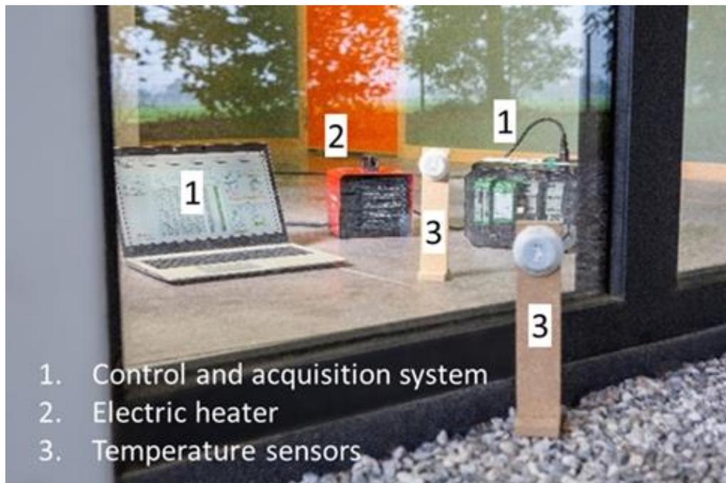
Figure 32. Equipment used in CoDY Test
