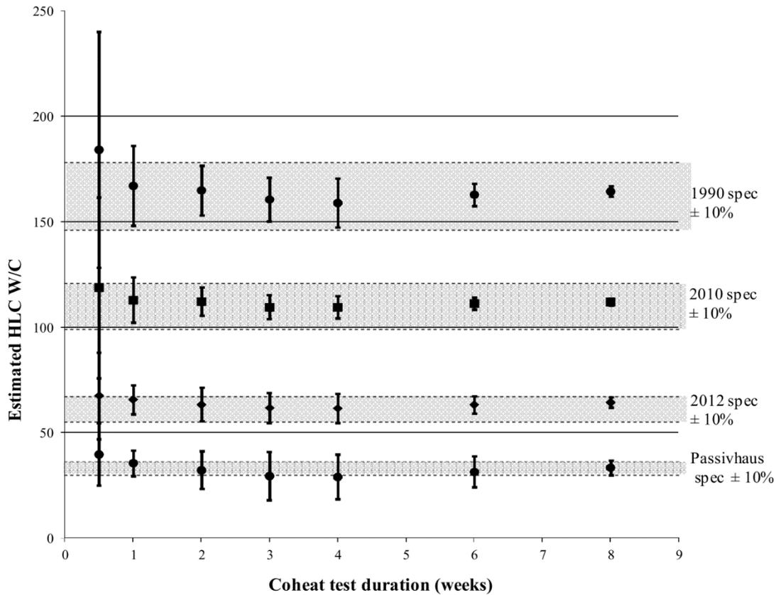
Figure 19. Coheating durations for different types of construction (Alexander and Jenkins, 2015)
