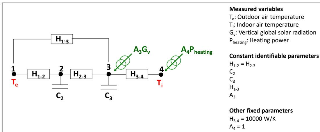
Figure 30. Model used to obtain the HTC of the RRTB.
