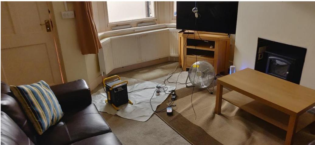
Figure 18. Coheating apparatus during a test
