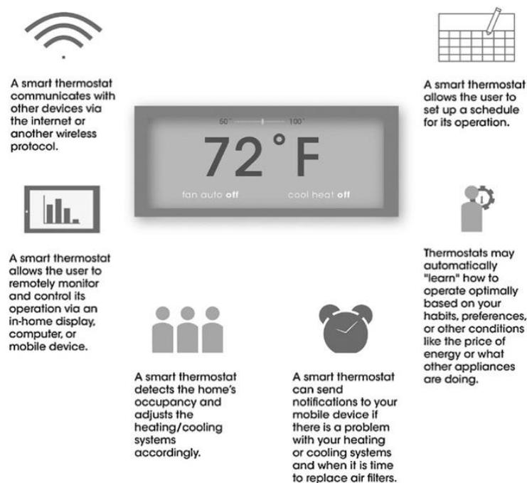
Figure 48. Typical facets of a smart thermostat (Sanguinetti et al., 2018)
