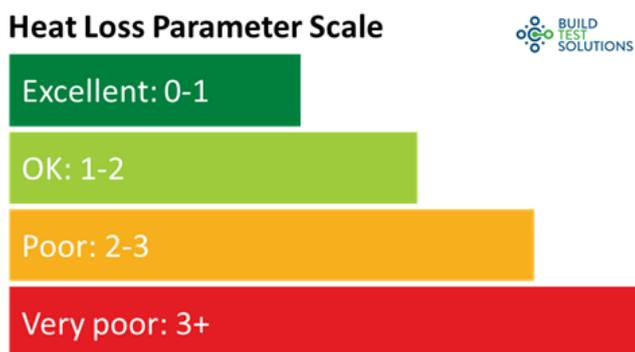
Figure 51. Example of HLP scale, provided by Build Test Solutions. <https://buildtestsolutions.com/heat-loss-parameter-a-metric-for-total-fabric-performance>
