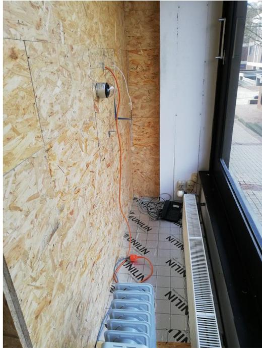
Figure 25. Temporary wall, Heating equipment and sensors used in CAM(B)BRIDGE Test
