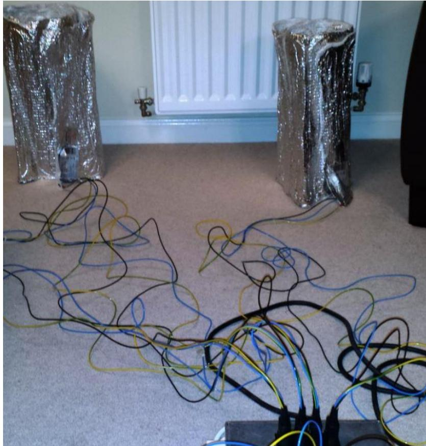
Figure 20. Heating equipment (foil mats) used in QUB Test
