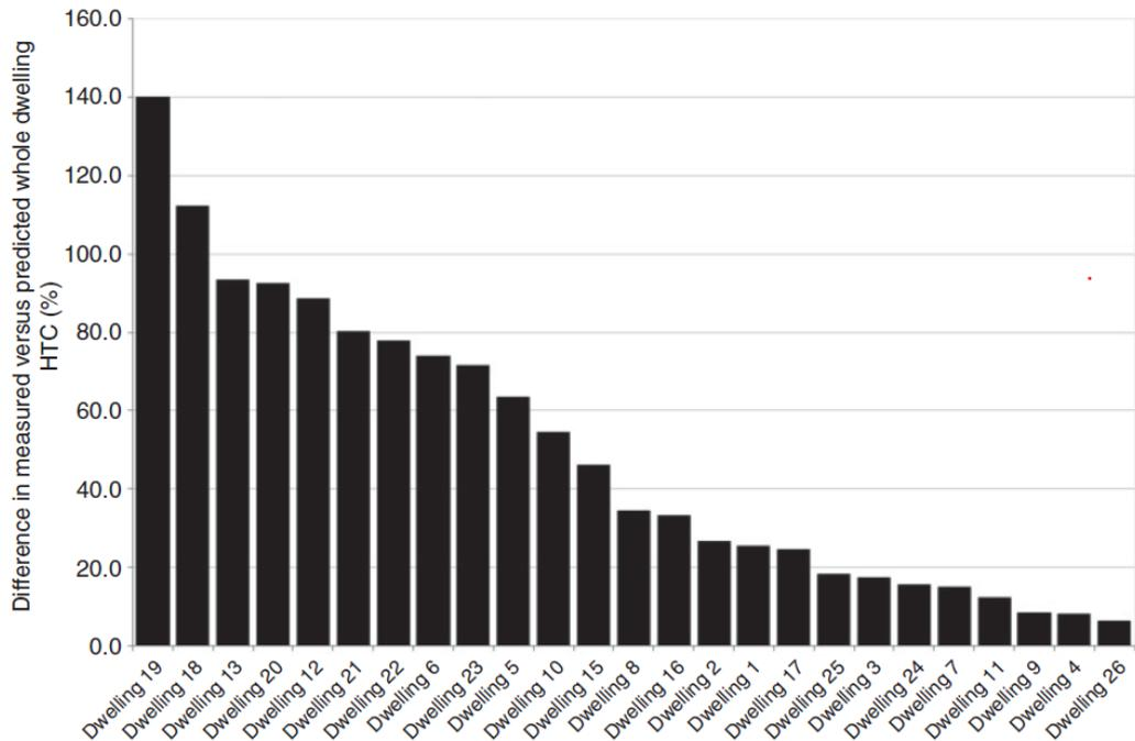
Figure 1. Results from a campaign of HTC (Heat Transfer Coefficient) measurement, illustrating the EPG in a sample of new build homes in the UK (D Johnston et al., 2015).
