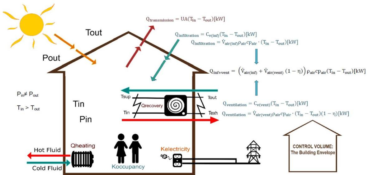
Figure 27. Schematic of all energy and mass exchanges through the control volume defined by the building envelope (Uriarte et al., 2019).
