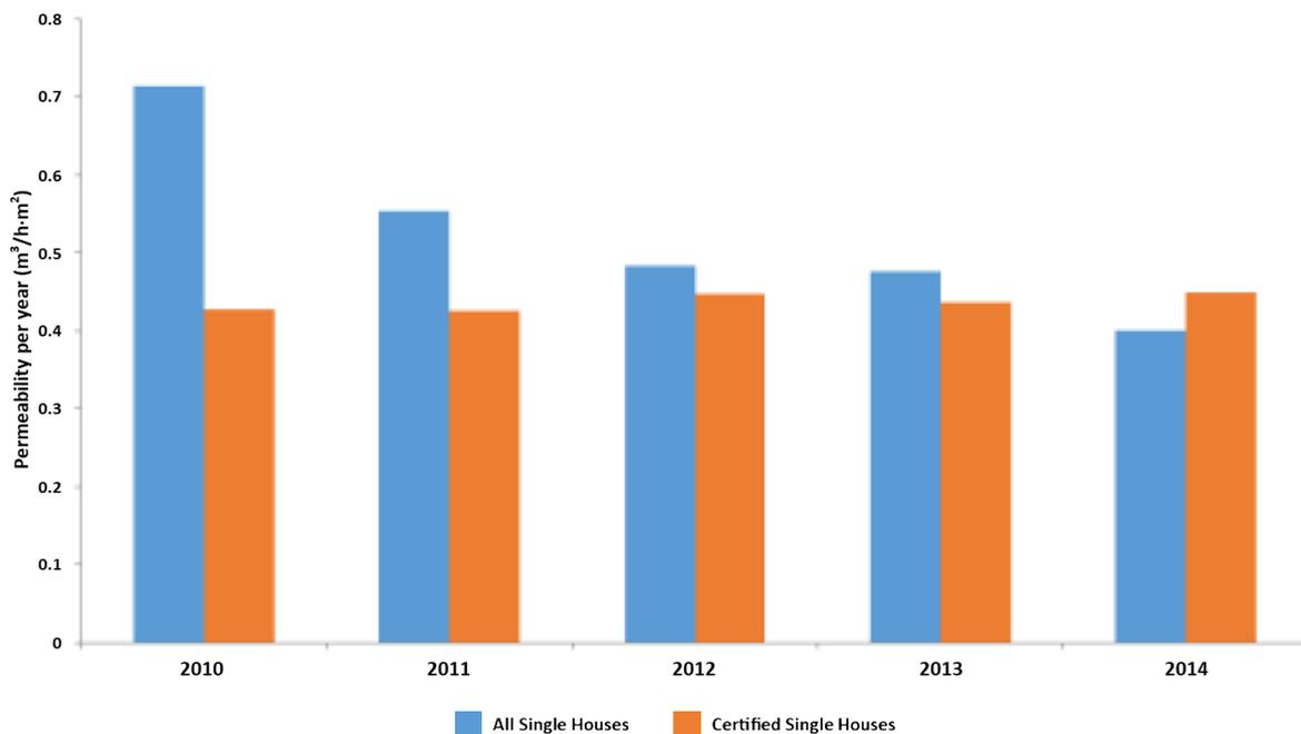
Figure 9. Average measured airtightness tendencies from 2010 to 2014 in France, for two samples of single-houses: a certified sample of single-houses and a control sample (not certified) (Observatoire BBC, 2015)
