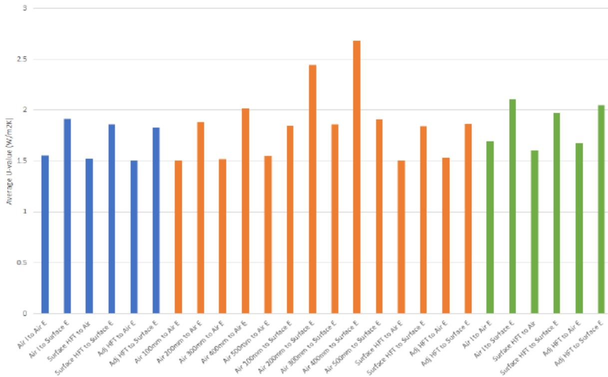
Figure 4. Illustrating the variation of U values across a simple wall. All measurements carried out on same wall area, with different temperature sensors placements and data analytics. Lowest U value = 1.5 W/m<sup>2</sup>K – Highest U Value = 2.6 W/m<sup>2</sup>K
