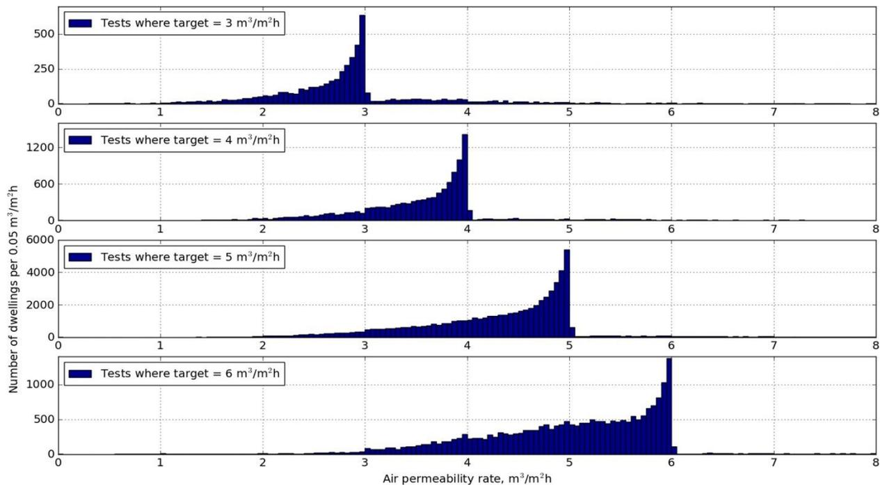
Figure 2. Results for sites with design targets of 3,4 5 and 6 m<sup>3</sup>/m<sup>2</sup>h. The design targets are the four most frequent in the dataset, representing 69% of the air permeability tests (Love et al., 2017).
