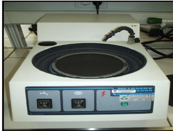
Figure 4.4: Metaserv 2000 Grinding Machine.
