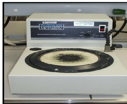
Figure 4.5: Polishing machine (Buehler Metaserv).
