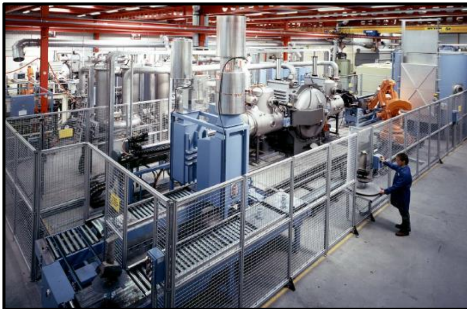
Figure 2.3: A modern high-volume production system for coating gas turbine blades-(Source: Sulzer).
