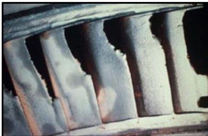
Figure 3.8: Erosion caused by corrosion in a jet engine gas turbine – [courtesy Boeing, USA ]
