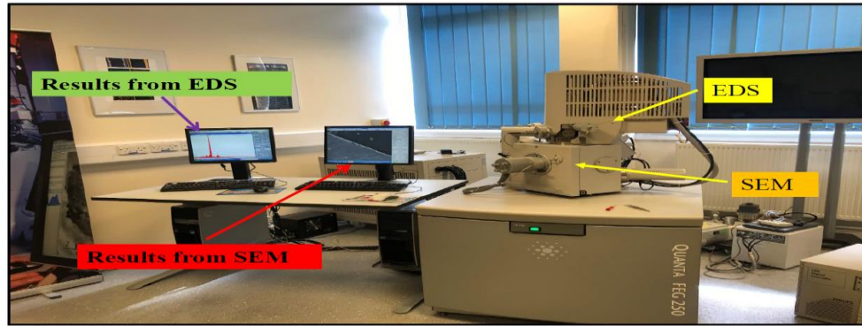
Figure 4.15: Scanning Electron Microscope and all other components [Quanta FEG 250, Germany].
