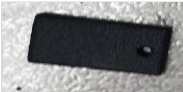
Figure 5.10: Nano-coated sample before TGA testing.
