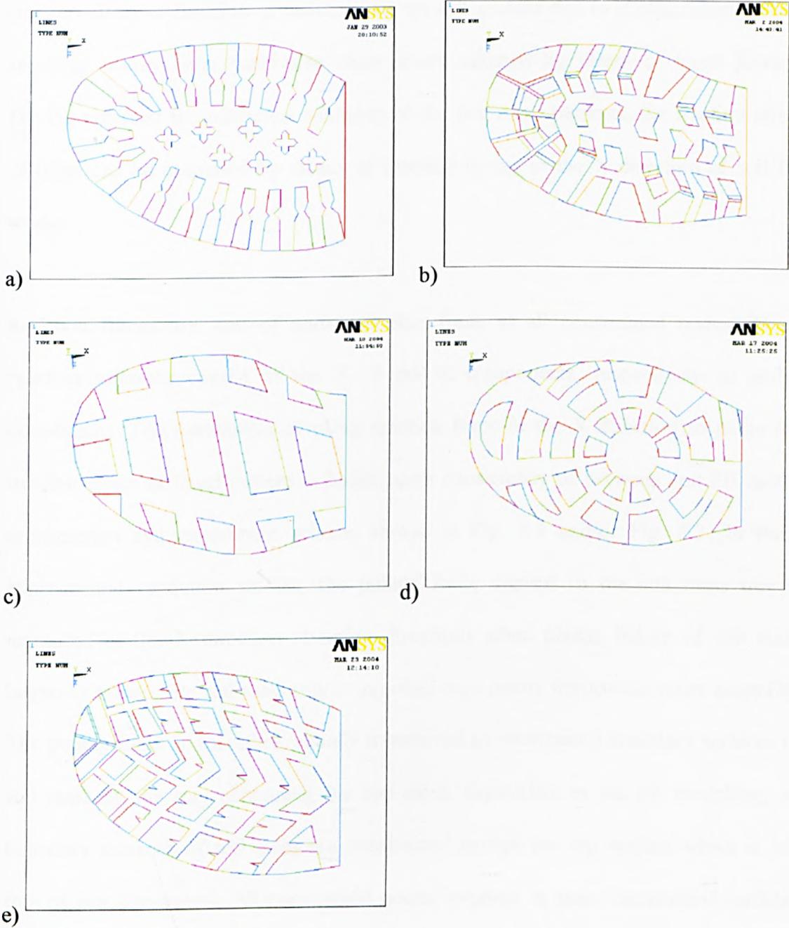
Fig. 6.29 The a) first, b) second, c) third, d) fourth, e) fifth tread patterns in plane
