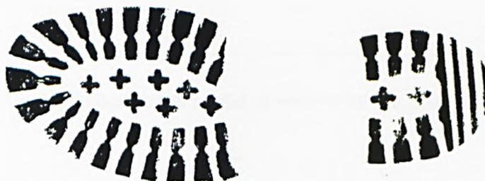
Fig. 6.4 Footprint of the first tread pattern
