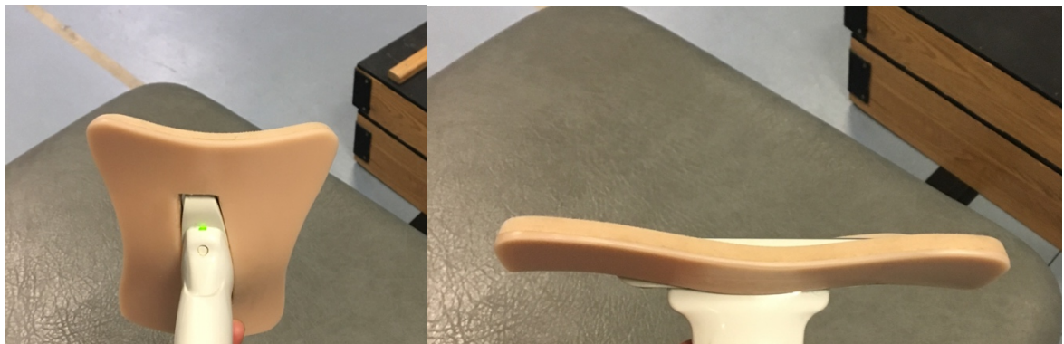
Figure 6-2 Custom designed cast, housing 10 cm ultrasound probe.
