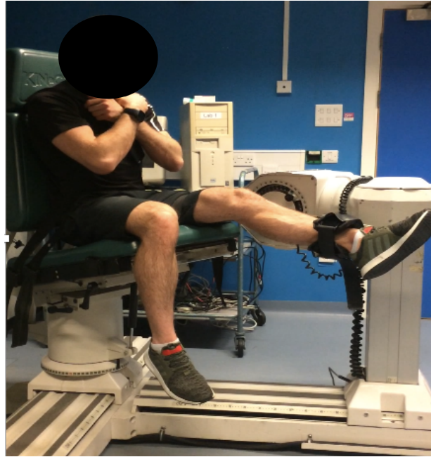
Figure 5-1 Image demonstrates the isokinetic dynamometry set up; current position represents measurement of limb weight at approximately full knee extension.
