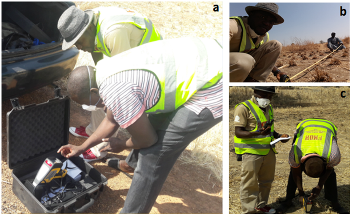
Figure 3. 5: Measuring the lead concentration on the four selected rice farms using the XRF Spectrometer (photo taken during the fieldwork).
