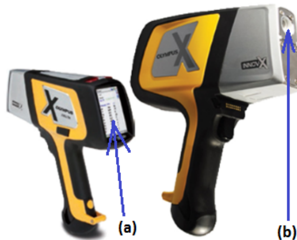
Figure 3. 2: Olympus Innov-X DELTA Professional XRF used for this study
