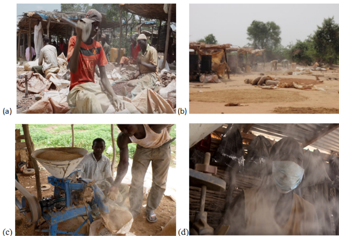
Figure 1.6: Crushing and grinding of the ore (Uriah et al., 2013; Udiba et al., 2012).
