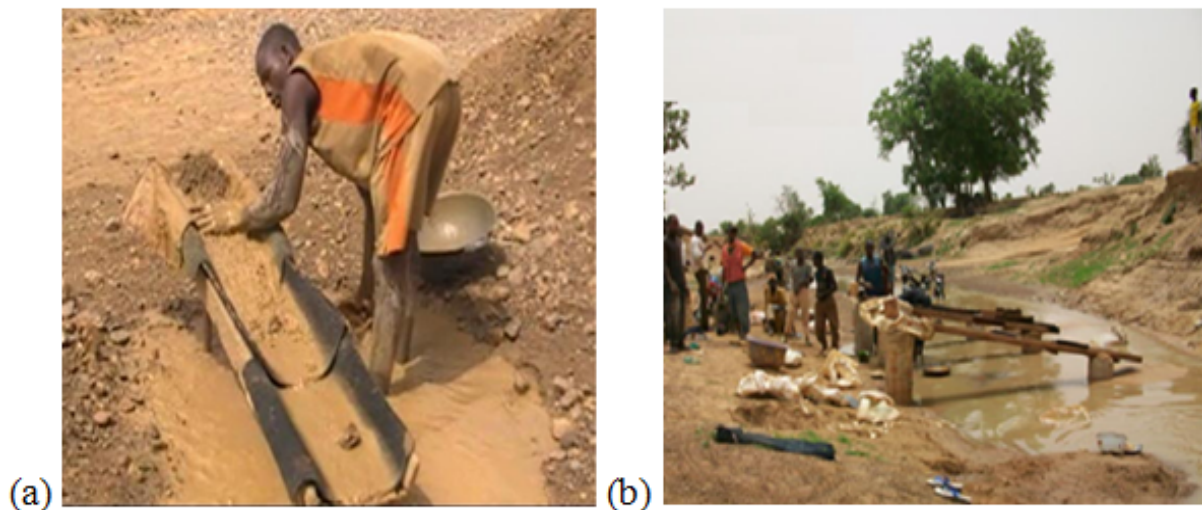
Figure 1.7: Using a locally made sluice box to wash the gold ore (photograph taken during the field work in 2017).
