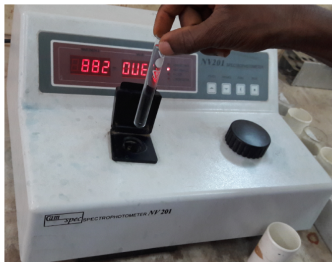
Figure 3.27: Spectrophotometer used to measure the available phosphorus in the soil samples
