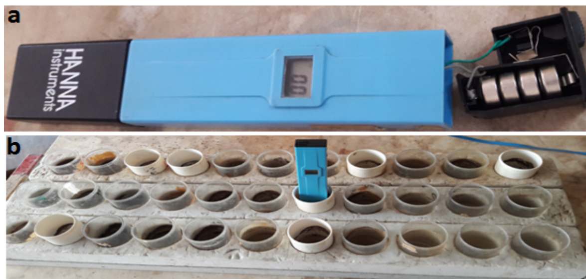
Figure 3.26: Electrical Conductivity meter
