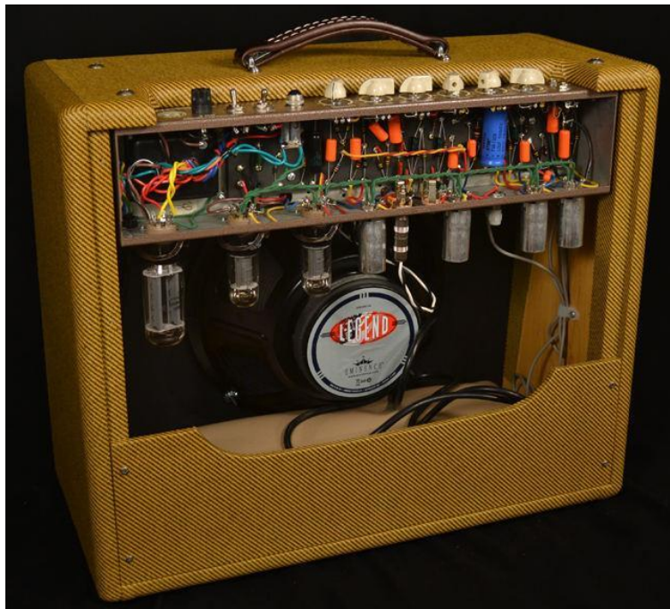
figure 13 Rear view showing the valve circuitry.
