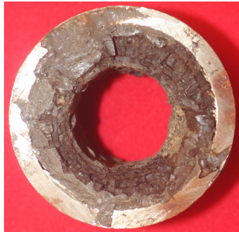
Figure 2: Cross section of wax deposit in production tubing.
