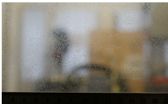
Figure 12. Impacted droplet deposition on glass test surface using sweeping action at the application distance of 1600mm ( L/D=6 )
