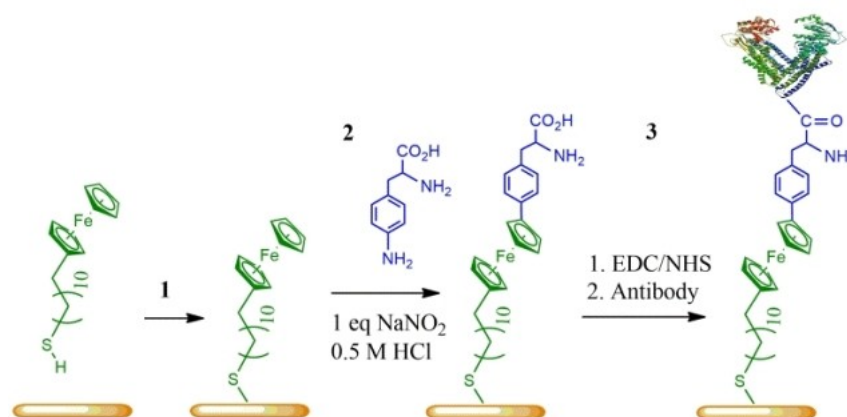
Scheme 1. Preparation of the sensing interface reported herein. Step 1: formation of the ferrocenethiol monolayer on a gold electrode. Step 2: grafting of amino-DL-phenylalanine onto the ferrocenethiol primer layer via in-situ formation of the corresponding diazonium cation. Step 3: Coupling of the receptive antibody onto the film.
