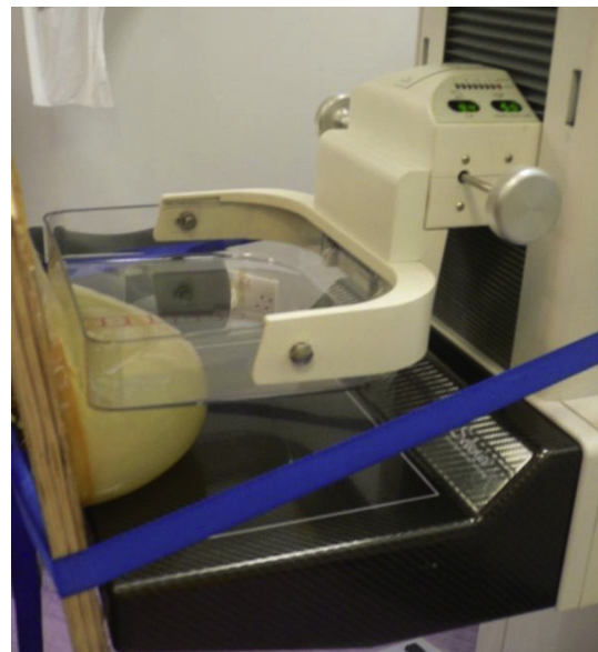
Figure 3. The experiment setup showing the breast phantom mounted semi-mobile onto a rigid supporting board.
