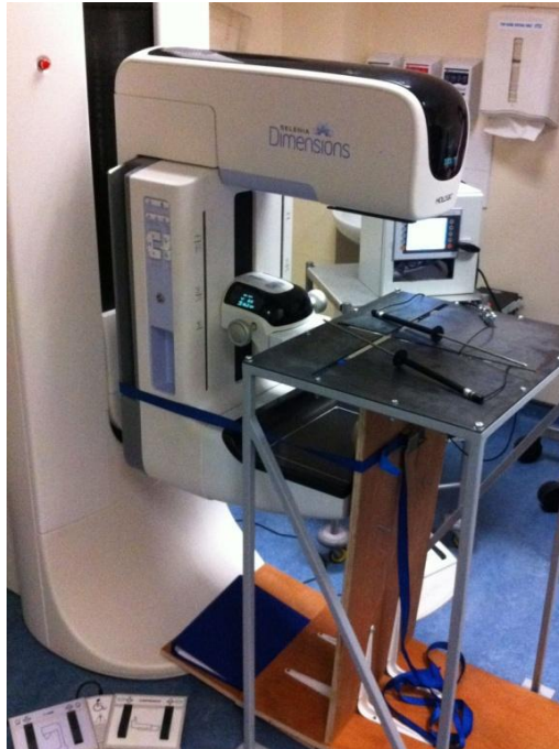
Figure 4. Deformable breast phantom mounted to rigid supporting board.
