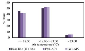
Figure 5. Annual effect of insulation on indoor temperature for SEH (base line U-Value=1.56 W/m<sup>2</sup>K).
