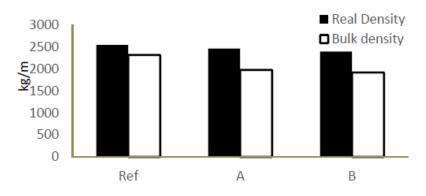
Figure 4 Density of concrete samples
