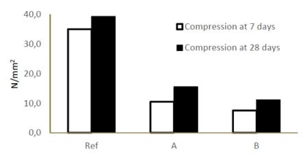
Figure 2 Compressive strength at 7 and 28 days
