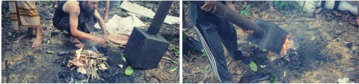
2 Fabricated metal reactor drilled with small holes and chimney placed over fire
