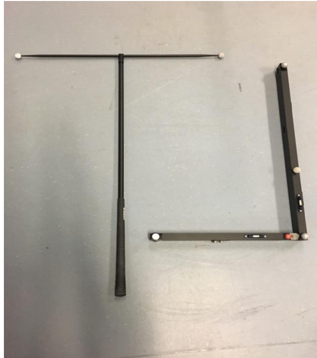
Figure 4-3 3D L-shaped frame and the T-shaped handheld wand for the Qualisys system.
