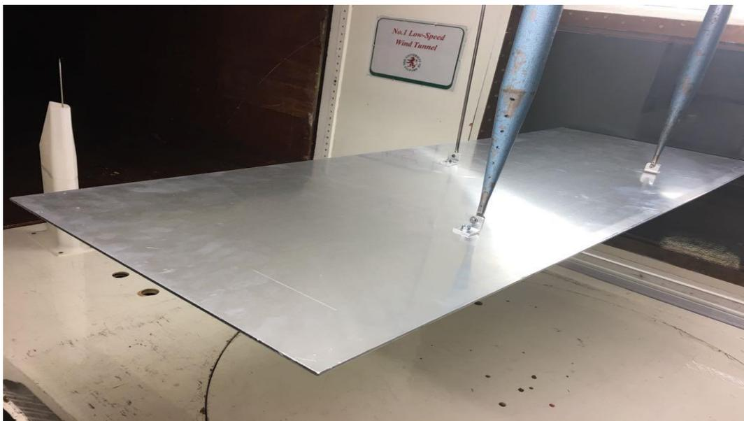
Figure 7.4 Struts to hold the flat plate in the wind tunnel
