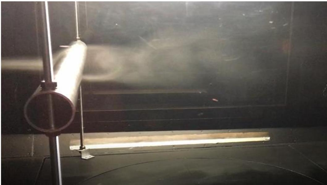
Figure 7.8 Smoke test for flow past a circular cylinder.
