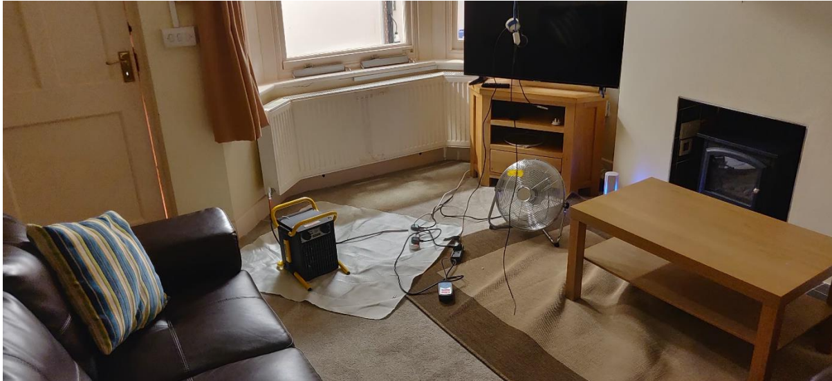
Figure 2 Image of Coheating test being performed.
