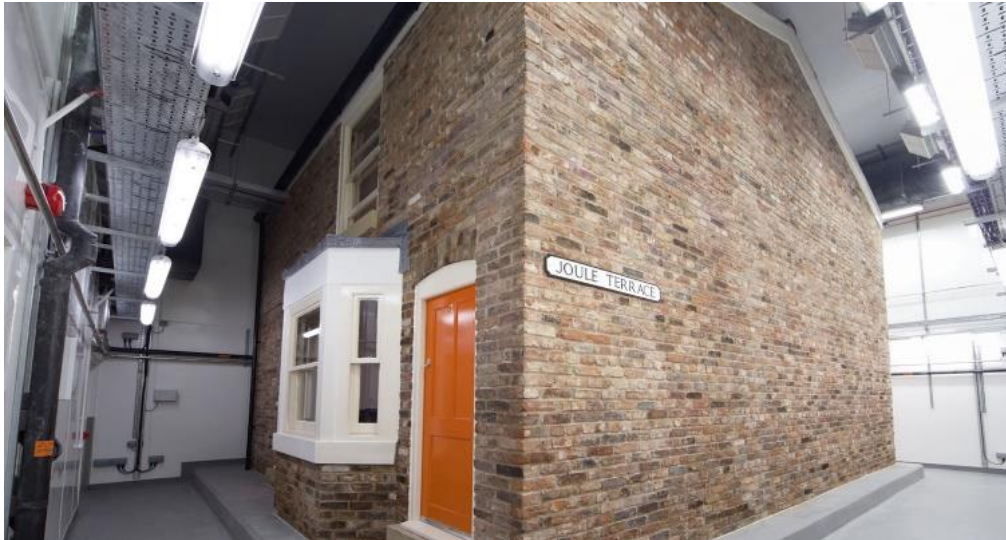
Figure 6 The Salford Energy House: A full scale end-terrace dwelling inside a climate-controlled chamber.
