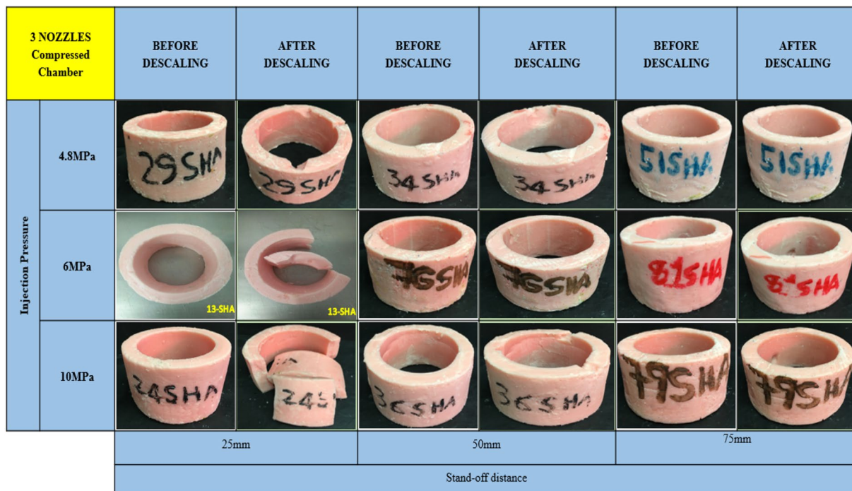
Fig. 21 Scale samples before and after descaling experiments with 3 nozzles (compressed chamber)
