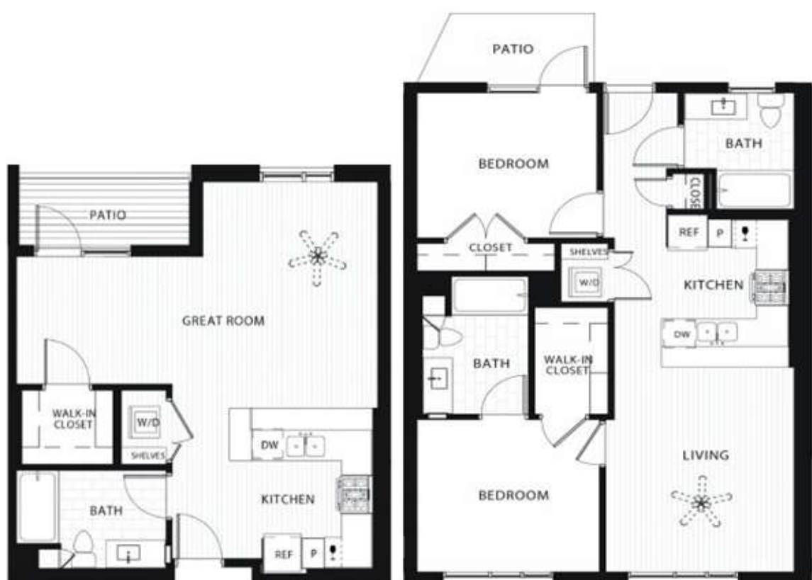
Figure 5.12: Floor plans for typical studio and two bedroomed apartments for a multi-family development (actual building shown in figure 5.13 below), Santa Monica City, Source: Developer's website: http://swaysantamonica.com/residences/floorplans , retrieved December 2018.
