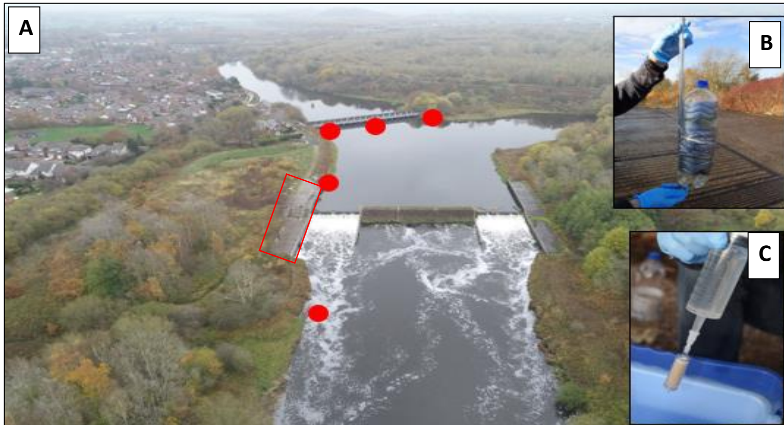
Figure 6: a) Sample locations (red dots) for the autumn sampling period and fish pass (red square) on Woolston weir; b) Water collection method attached to the pole (top right); c) Filtering method with syringe (bottom right).
