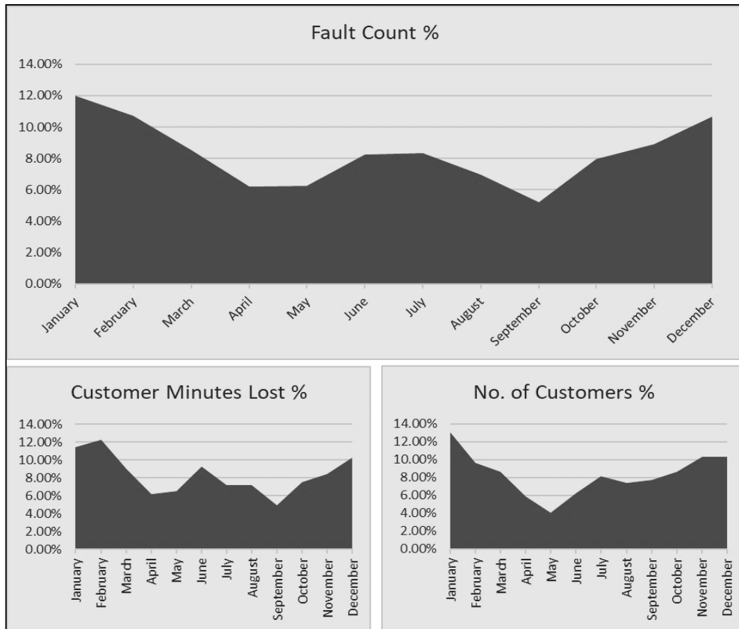
Figure 5.2: Average monthly changes in faults due to equipment failures in the Ausgrid case study
