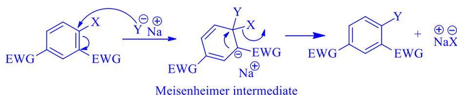
Scheme 13: addition-elimination nucleophilic substitution mechanism  $S_NAr$  (Goldstein *et al.*, 2017).
