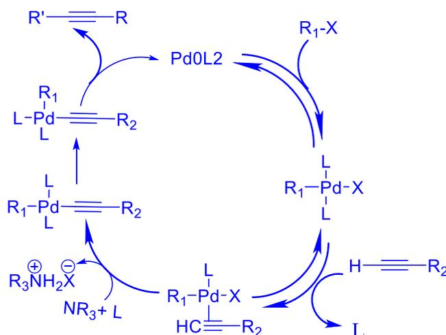
Scheme 4: Proposed copper-free Sonogashira coupling mechanism (Mery *et al.*, 2003).
