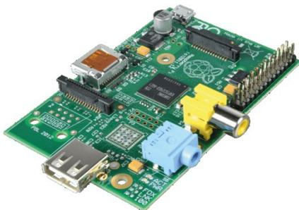
Figure 2.3 Raspberry Pi (Raspberry Pi, 2016)
