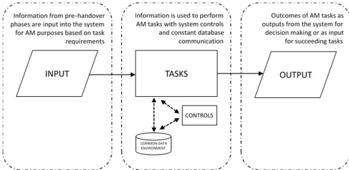
Figure 6: BIM-based AM Input-Output system
