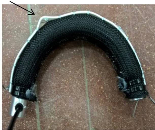
**Figure 2.** The structure of the self-bending contraction actuator version I. (a) The layout of the reinforcement rod. (b) The bending actuator after several operations.
