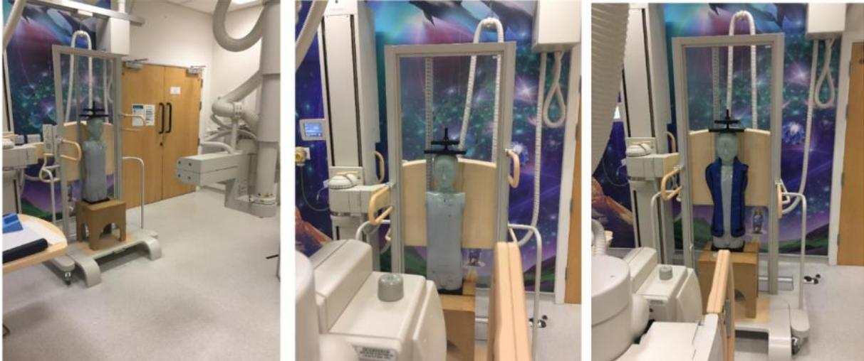
Figure 3.13: The phantom positioned for DR imaging.
