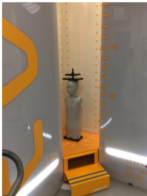
Figure 3.14: The phantom in the EOS imaging system.
