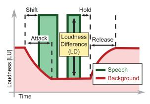
Fig. 1. Ducking of the background while foreground speech is active. This is controlled by parameters such as the Loudness Difference (LD) between speech and background during ducking and time constants (attack, shift, hold, release).
