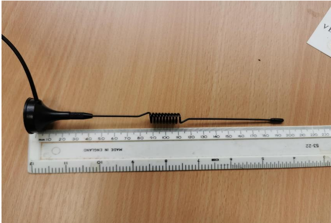
213. Figure (25): One of the helix monopoles utilised for gain measurements
