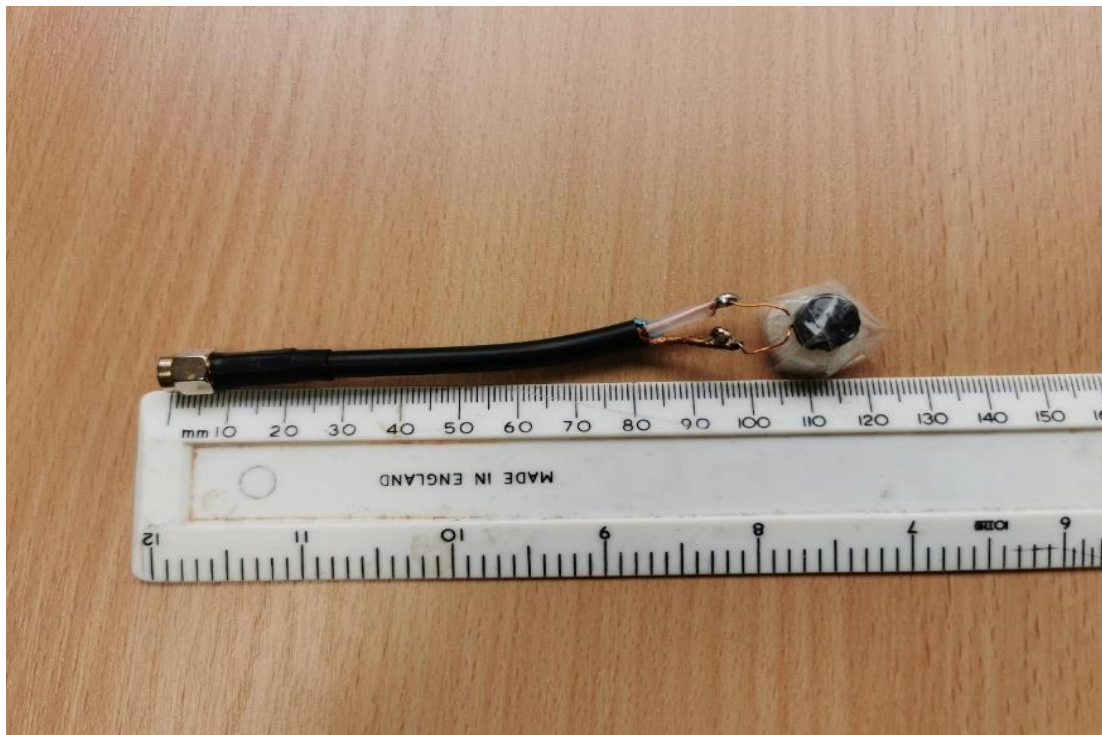
214. Figure (26): The copper 8.5 mm OD on ferrite substrate, with plastic fixer cap
