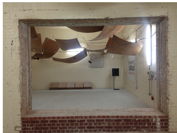
Figure 3.2: Large reverberant room ( 5s RT_{60} )
