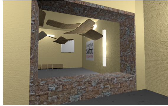
Figure 4.12: VE large reverberant room ( 5s RT_{60} )
