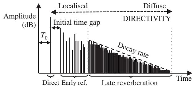
Fig. 1. Generic RIR model (based on [10], Fig. 1), showing the squared magnitude. Direct sound arrives after time  $T_0$ , early reflections begin after the initial time gap, and late reverberation decays exponentially. Sound becomes increasingly diffuse with time.
