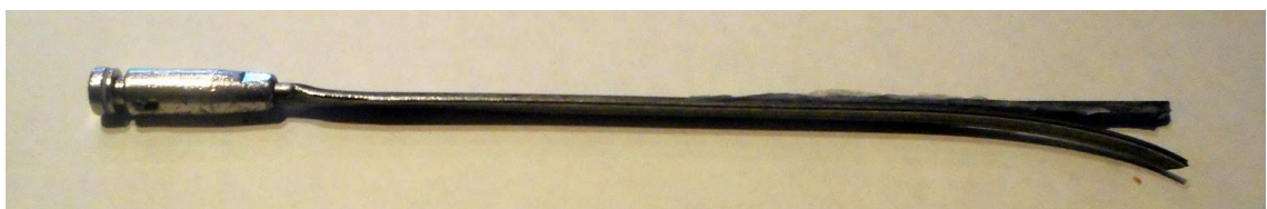
Figure 2 – Tip of broken blade [87].
