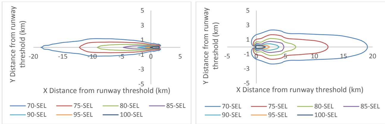
Figure 1: SEL contours of the Airbus A320-232 aircraft at arrivals (left) and departure (right).
