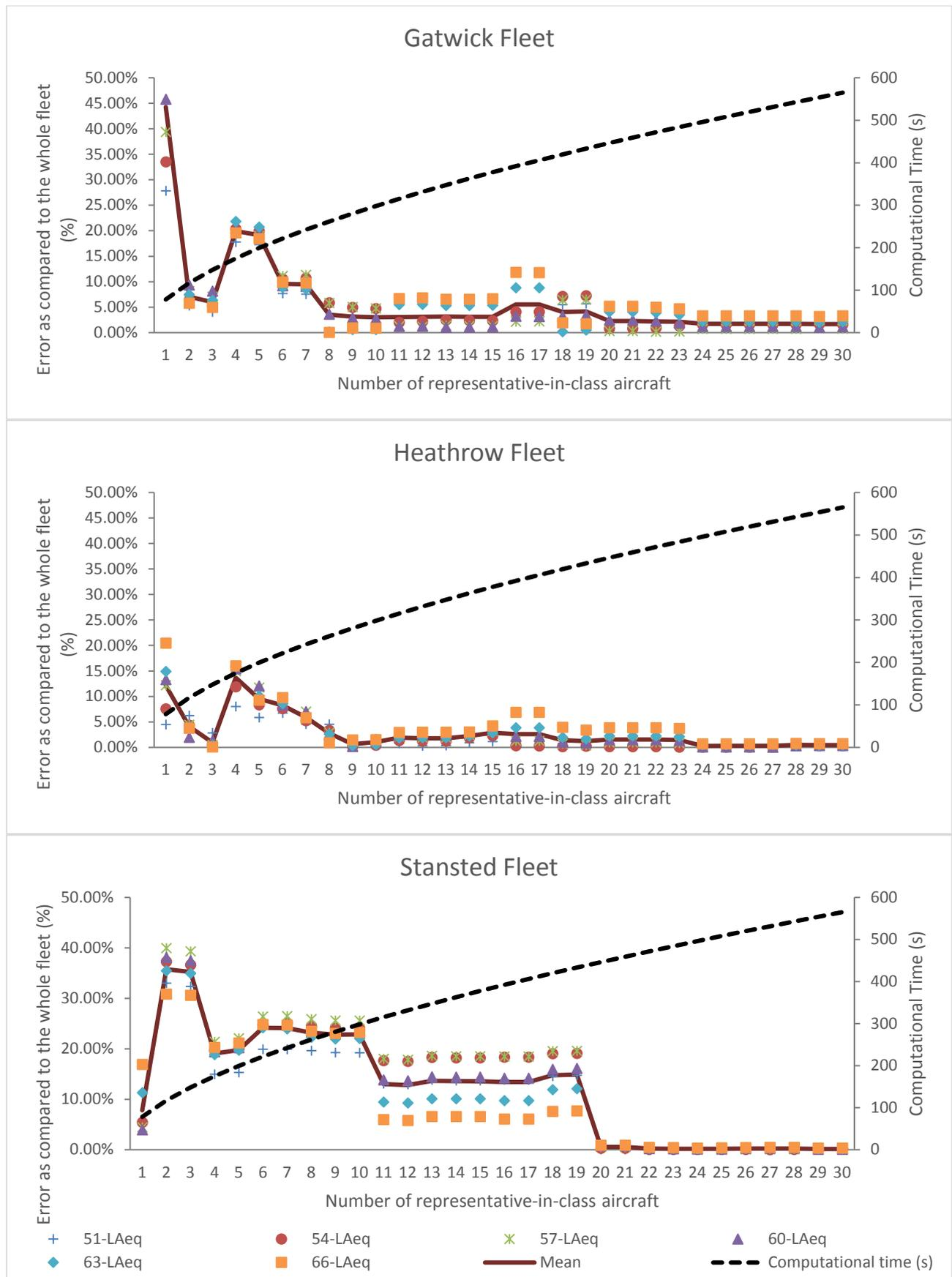
Figure 2: Relative error of the calculation of noise contour areas when a number of representative-in-class ( $n = [1, \dots, 30]$ ) replaces the whole aircraft fleet aircraft and the associated computational time, for the Gatwick (top), Heathrow (middle) and Stansted (bottom) aircraft fleet in 2015.
