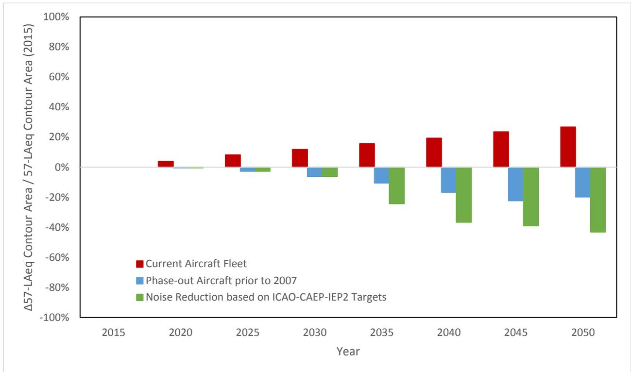
Figure 3: Change in 57-L<sub>Aeq,16h</sub> noise contour area in the UK for the period 2015-2050, without novel aircraft technologies (red bars), retiring all aircraft produced before 2007 (blue bars) and introducing new aircraft (in 2030) meeting ICAO-CAEP-IEP2 targets [14].
