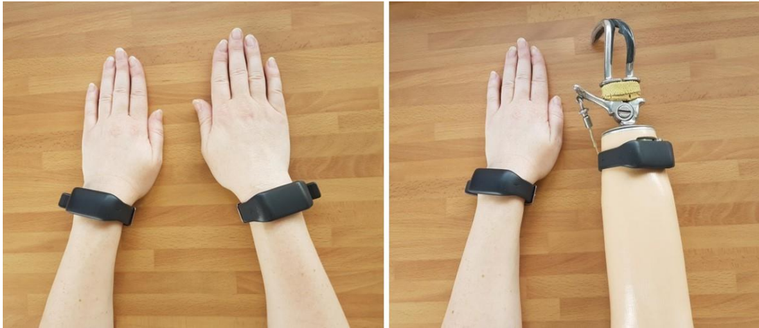
Figure 15: How devices are worn on anatomically intact and limb absent participants. Left: anatomically intact Right: upper limb absent (author's own image)
