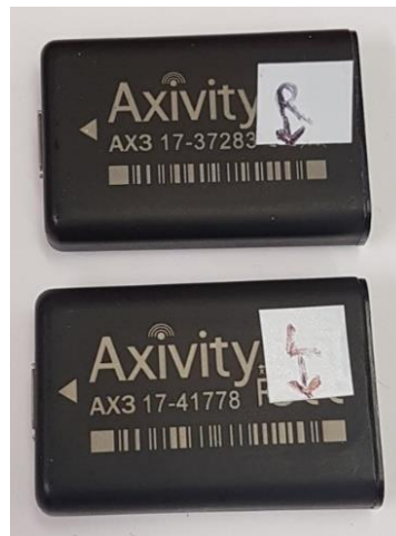
Figure 14: Labelled devices to indicate side to be worn on and correct orientation (author's own image)
