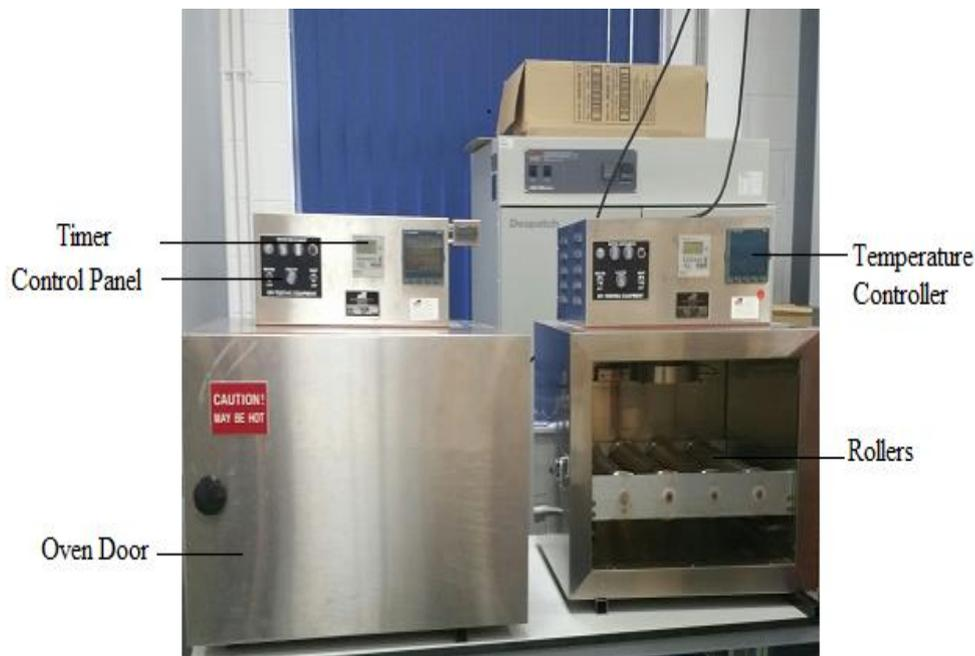
**Figure 4.8:** The 4-roller oven and the 5-roller oven
