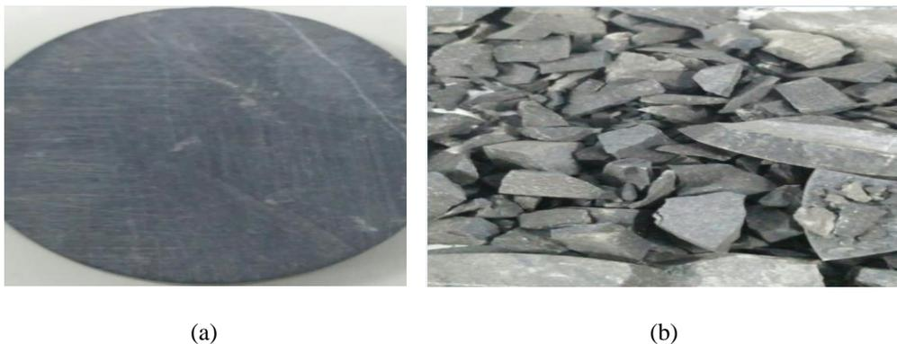
**Figure 4.10:** Photo images of Marcellus shale samples: (a) Surface of dried shale plug; (b) Dried shale cuttings
