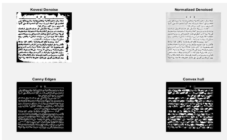
Figure 5-5 Example of the steps used in the Noise removal phase
