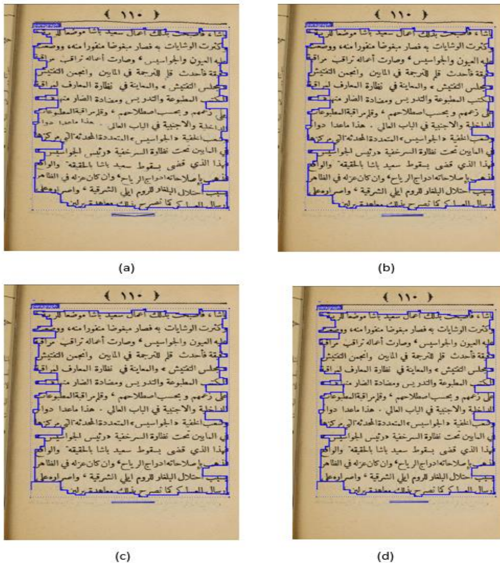
Figure 6-3 (a) authentic image (b) dewarped image by coarse dewarping (c) Book-Restorer results (d) dewarped image by ground truth dewarping
