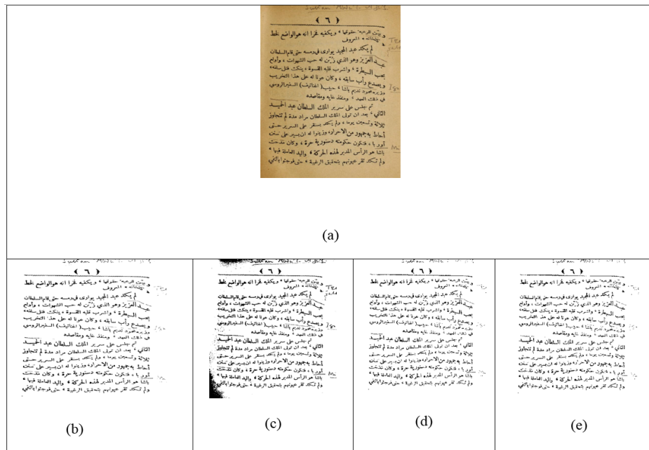
Figure 5-4 Sample warped document images image: (a) An original warped image, (b) after applying Sauvola binarisation, (c) after applying threshold (d) after applying Otsu binarisation, (e) after applying Phase-Based Binarisation
